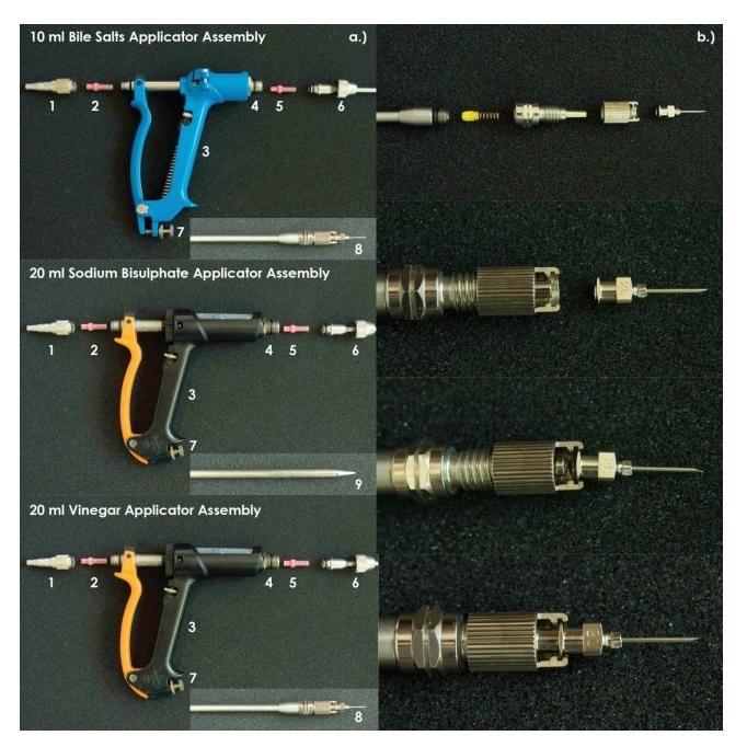
Figure 1 Assembly of the three applicators. a) 1: inlet adaptor, 2: inlet valve assembly, 3: hand piece, 4: delivery valve cage, 5: delivery valve assembly, 6: spear nut, 7: dose adjustor screw, 8: lock nut and veterinary needle, 9: tip of the spear of the sodium bisulphate applicator; b) Step-by-step sequence showing the correct assembly of the lock nut and the veterinary needle used in the bile salts and vinegar applicators. © Daniel Schultz
