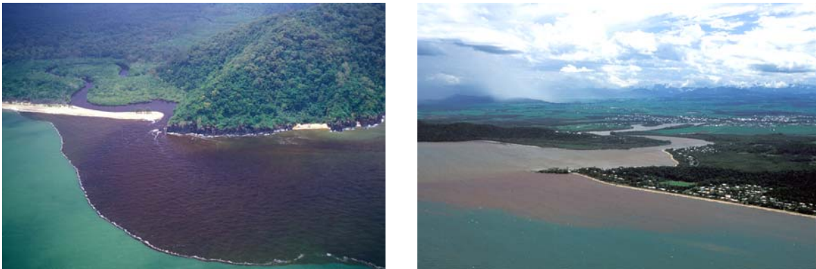
Figure 3: Comparison of flood plumes from a pristine catchment (left) and a developed catchment (right) Photographs © Great Barrier Reef Marine Park Authority
