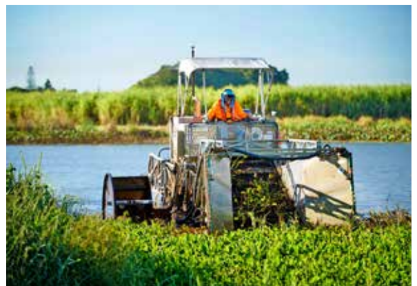
Taking action: water weeds officer using a weed harvester to remove aquatic weed in Lilliesmere Lagoon
