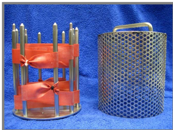
Figure 3.5. PDMS passive samplers loaded onto stainless steel sampler supports which sits within the deployment cage and is sealed in place with wing nuts
