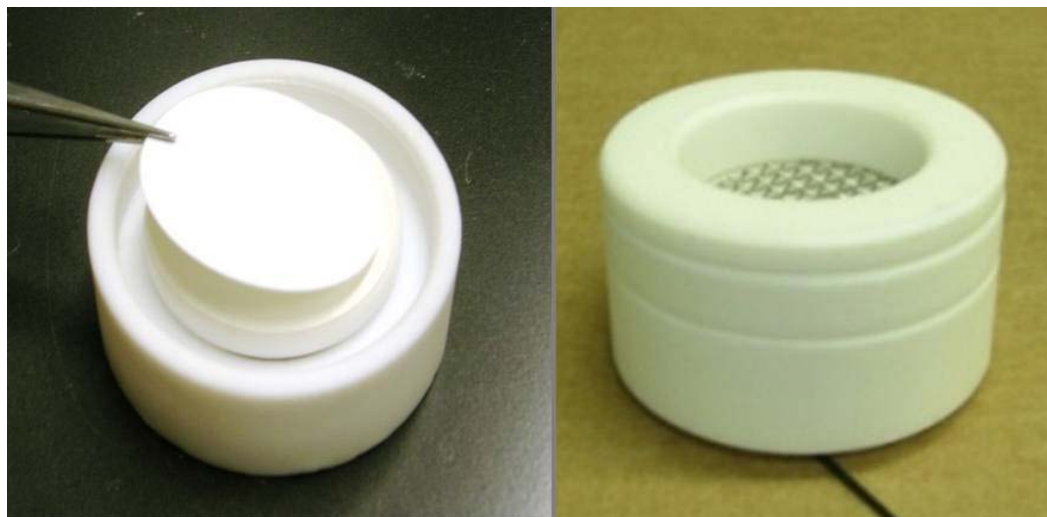
Figure 3.2. An Empore disk (ED) being loaded into the Teflon Chemcatcher housing (LHS) and an assembled housing ready for deployment (RHS).
