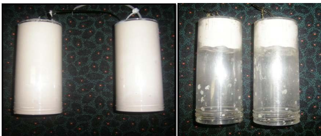
Figure 3.3. Passive flow monitors (PFMs) prior to deployment (LHS) and post-deployment (RHS)
