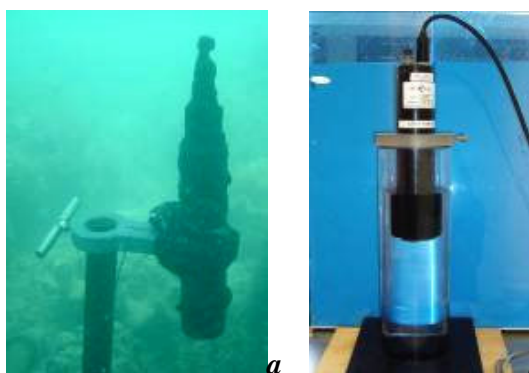
Figure 4.16. Wet Labs FLNTU combined chlorophyll a and turbidity logger a) Logger deployed at Dunk Island (wrapped in plastic for protection) b) Logger immersed in calibration chamber.
