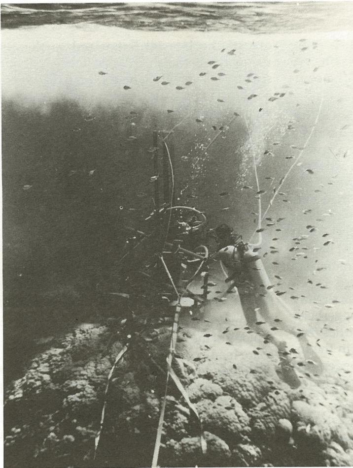
*AIMS scientist coring corals with a drilling rig especially designed and built by the Institute.. Photo courtesy AIMS*
