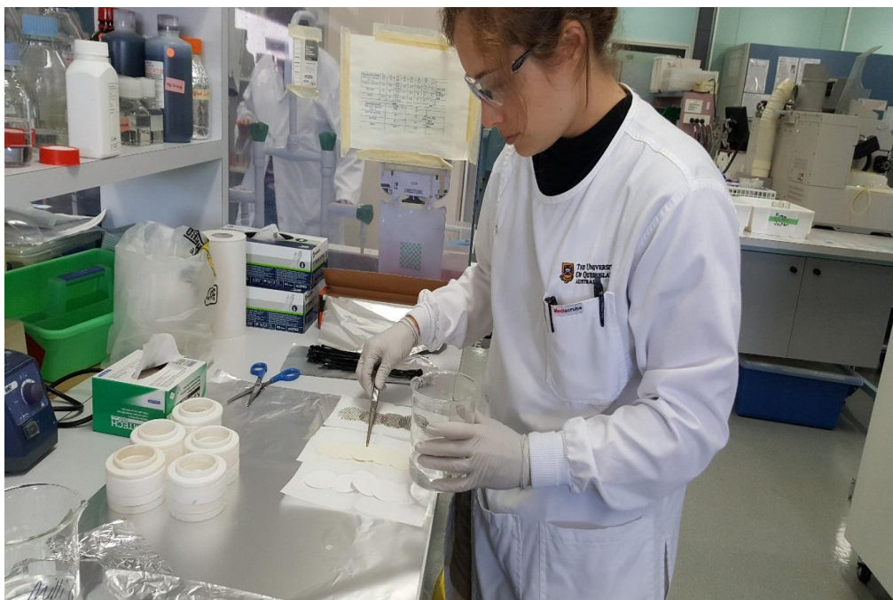
Figure 3. Preparation of an Empore disk (ED) passive sampler.
