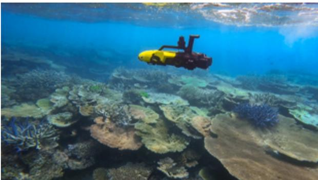
The RangerBot underwater drone and ASVs (equipped with GoPro cameras) conducted coral mapping transects and manta tow surveys for detecting crown-of-thorns starfish (COTS).
