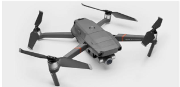
The DJI Mavic aerial drone conducted aerial mapping to collect orthomosaic images. High resolution images were gathered at 115, 100, 80, 60, 40 and 20m altitude.
