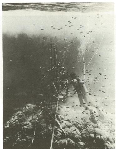
AIMS scientist coring corals with a drilling rig especially designed and built by the Institute.. Photo courtesy AIMS
