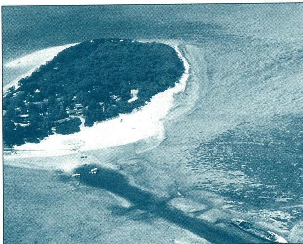
**Photo 1.** Heron Island harbour channel in 1979, prior to the construction of bund walls. Large erosion scars are evident as a result of water draining through the channel at low tide.
