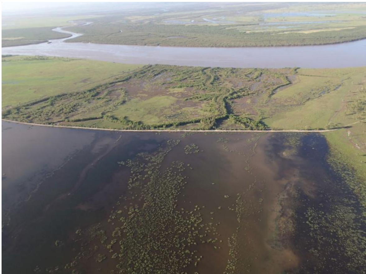
Figure 11: Poned pasture on northern bank at mouth of Fitzroy River effectively acting as a barrage on tributaries of the river. Location shown in Figure 9 and Figure 10. Photograph by Jim Tait (2013)
