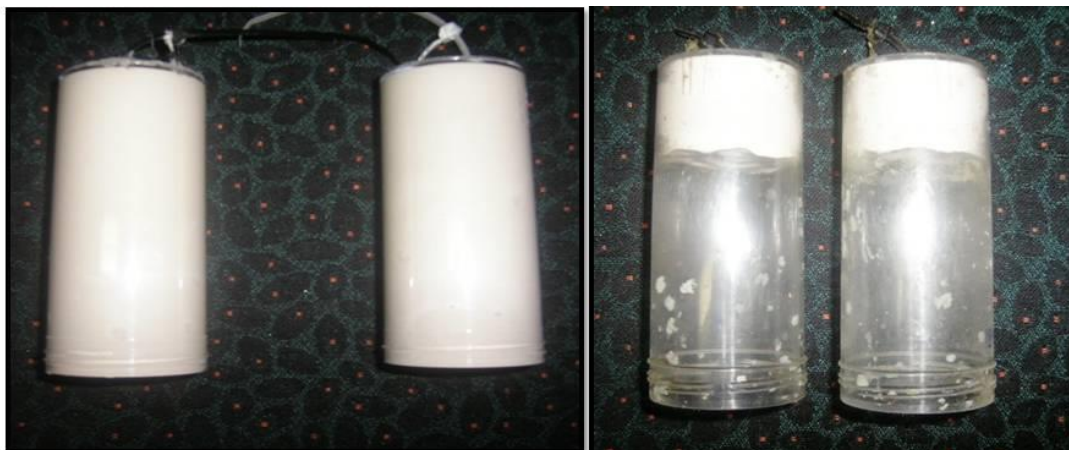
Figure 4-2 Passive flow monitors pre-deployment (left) and post-deployment (right)
