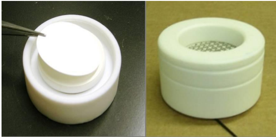
Figure 4-1 An Empore Disk being loaded into the Teflon Chemcatcher housing (left) and an assembled housing ready for deployment (right)
