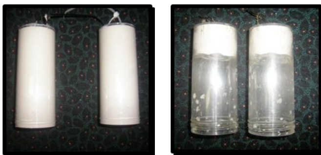
Figure 2-4: Passive flow monitors (PFMs) prior to deployment (left) and after deployment (right).
