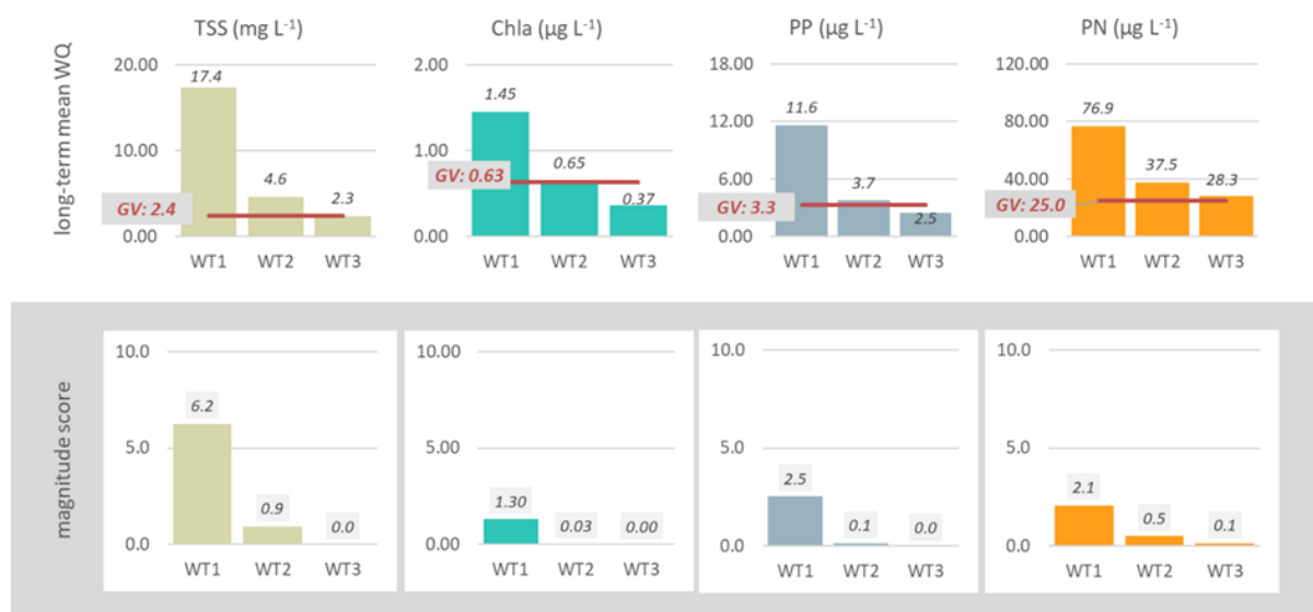
Figure 3-6: Mean long-term concentrations of water quality parameters (top) and magnitude scores across the three Reef water types (bottom). Red lines show the Reef-wide wet season GV’s (Table 3-3). Magnitude scores are calculated as the proportional exceedance of the guideline: magnitude_{water\ type} = ([Poll.]_{water\ type} - GV)/GV and Poll. = TSS, Chl-a, PP, \text{ or } PN . Negative magnitude scores are scored as zero.
