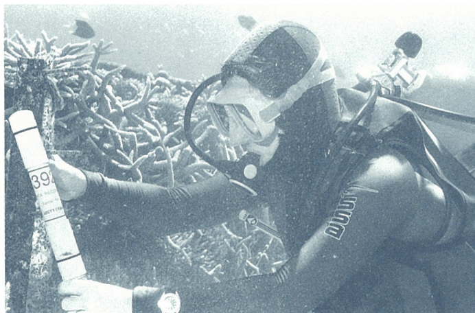
Left: Continuously recording temperature loggers are deployed at representative sites in the Great Barrier Reef Marine Park to help staff understand major natural events on coral reefs such as coral bleaching.
