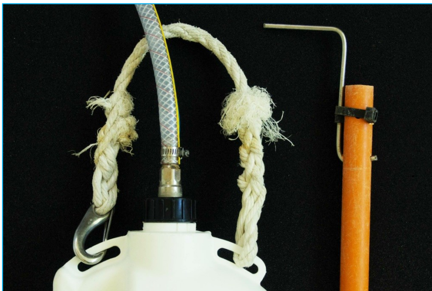
Figure 3 Hook and bottle with spliced rope and clip. © Daniel Schultz
