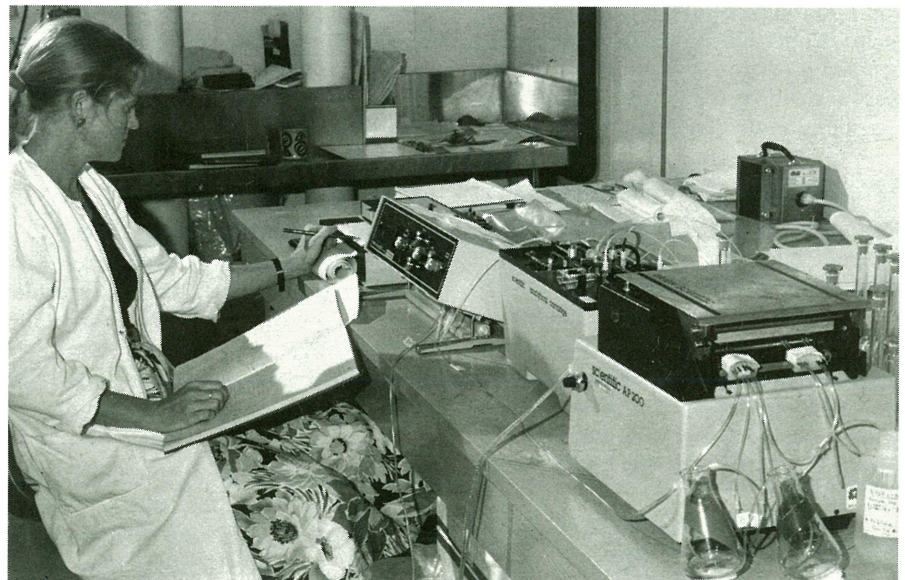
Control of water quality requires regular measurements of nutrients. Biologist Dr Janice Morrissey uses an auto-analyser to test tank water samples.
