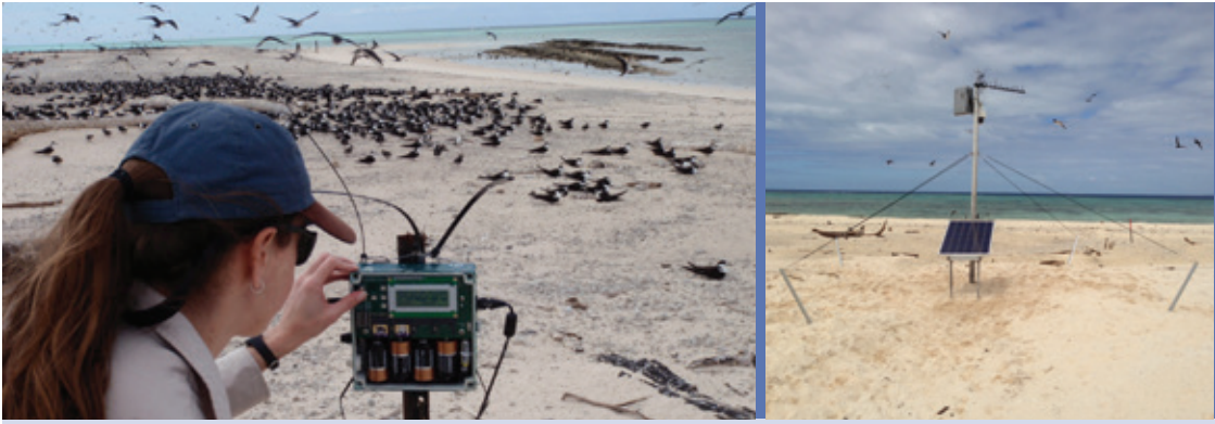
Left: A field management ranger checks the acoustic monitors on Michaelmas Cay. Right: The pole-mounted video camera which takes continuous high-definition footage on Michaelmas Cay. Photographs courtesy of Queensland Parks and Wildlife Service.
