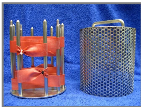
Figure 4-7 PDMS passive samplers loaded onto stainless steel sampler supports which sits within the deployment cage and is sealed in place with wing nuts
