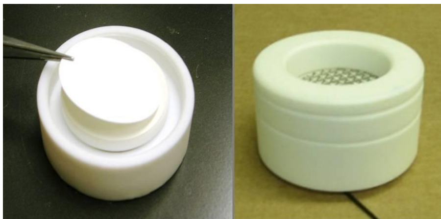
Figure 4-2 An Empore disk (ED) being loaded into the Teflon Chemcatcher housing (LHS) and an assembled housing ready for deployment (RHS)
