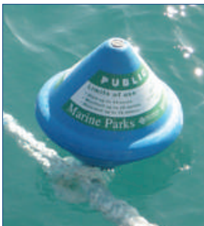
Public mooring buoy - this illustrates a B class mooring
