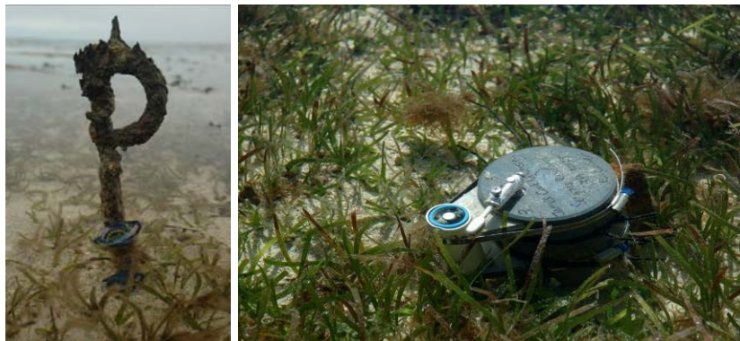
Autonomous iBTag™ submersible temperature loggers and submersible Odyssey™ photosynthetic irradiance autonomous logger deployed at Green Island.
