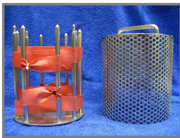
Figure 4-5 PDMS passive samplers loaded onto stainless steel sampler supports which sits within the deployment cage and is sealed in place with wing nuts
