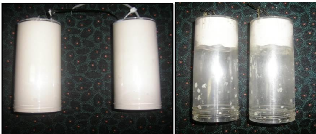
Figure 4-3 Passive flow monitors (PFMs) prior to deployment (LHS) and post-deployment (RHS)
