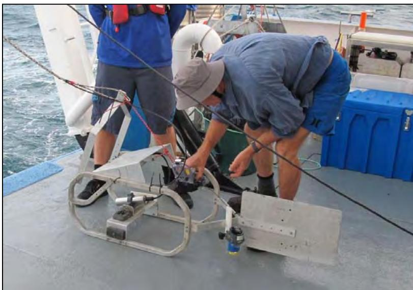
Figure 2. Towed underwater video equipment on the rear deck of the *RV Cape Ferguson*
