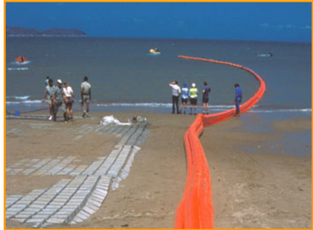
A boom being deployed near Townsville to deflect and contain oil during a training exercise. Training in the use of all oil spill combat equipment and response management is vital for effective oil spill response.
