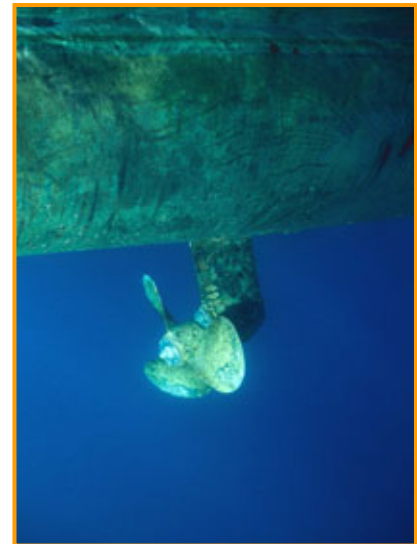
Hull fouling is a potential vector for the spread of pests. Organisms settle on the hull, propeller, sea chests and other parts of ships and are transported to other sites where they may become a pest.
