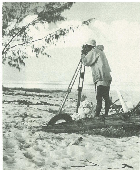
An officer of the Australian Survey Office establishing one of the reference points for accurate position fixing of their dinghy which is used for obtaining echosounding profiles.
