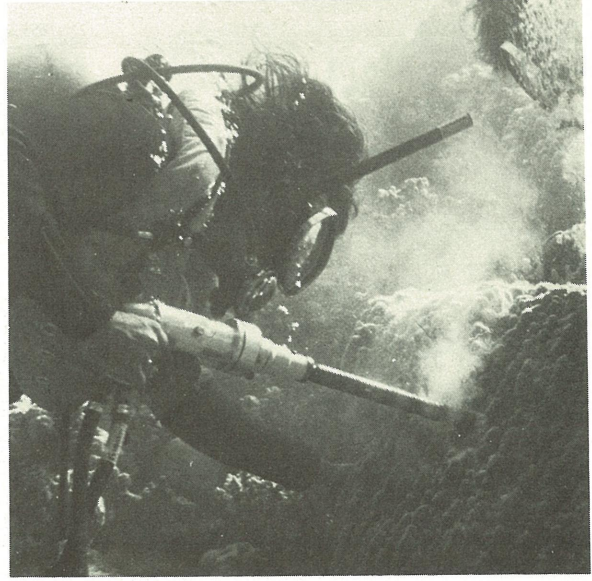
A researcher from James Cook University sampling a Porites head for radio-metric dating, using an air-driven coring drill which takes cores of up to 1 metre in depth. Photograph: J. Barnett
