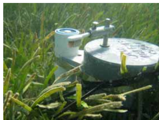
A functioning lightlogger recording conditions in a seagrass meadow
