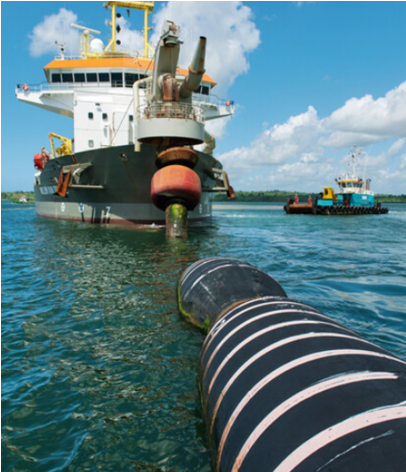
Trailing suction hopper dredge and floating pipeline.
