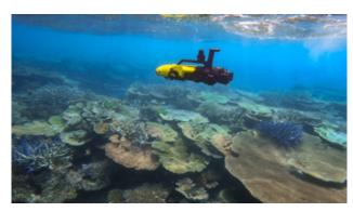
The RangerBot underwater drone and ASVs (equipped with GoPro cameras) conducted coral mapping transects and manta tow surveys for detecting crown-of-thorns starfish (COTS).
