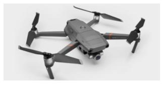
The DJI Mavic aerial drone conducted aerial mapping to collect orthomosaic images. High resolution images were gathered at 115, 100, 80, 60, 40 and 20m altitude.
