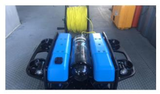
The BlueROV underwater drone conducted a visual assessment of a mooring line.
