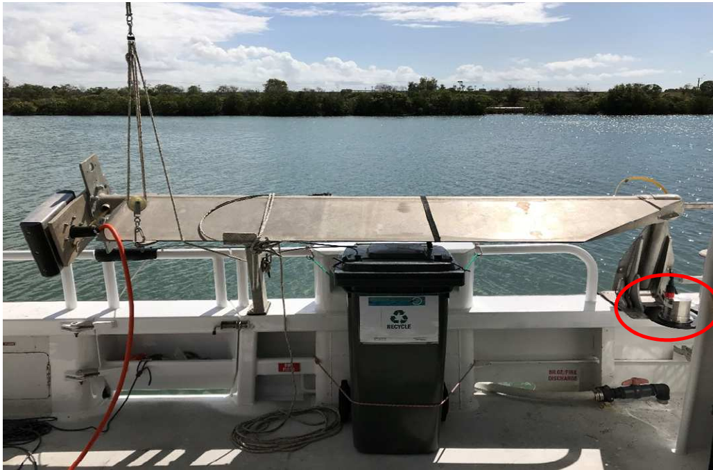
Figure 12: Mounting pole on WILD BLUE. POS MV IMU located inboard of pole on an AI supplied plate. SES-2000 SBP transducer attached to an adaptor flange connected to the R2Sonic flange associated with pole.
