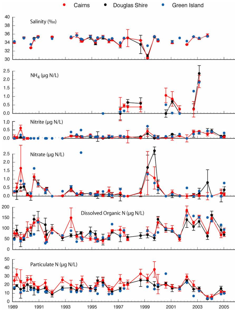
Figure 3.7 Median values of depth-weighted average water column salinities and concentrations of fixed nitrogen species in coastal and lagoonal waters off Douglas Shire (4 sites), Cairns (5 sites) and Green Island (1 site) between April 1989 and January 2005. Error bars for the pooled stations off Douglas Shire and Cairns show the 95% confidence range for these sites.
