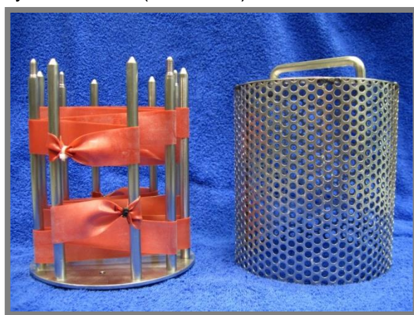
Figure 3.5. PDMS passive samplers loaded onto stainless steel sampler supports which sits within the deployment cage and is sealed in place with wing nuts
