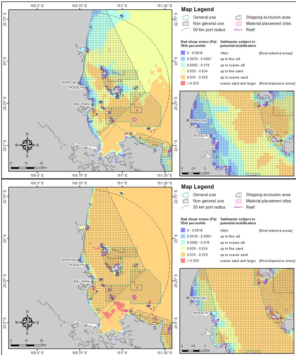
**Figure 29.** Distribution of the 50<sup>th</sup> (upper) and 95<sup>th</sup> (lower image) percentile bed shear-stress estimates within 50 km from Rosslyn Bay State Boat Harbour. The estimates were calculated at hourly steps for each grid cell during 2011 current and wave conditions. The insets show a close-up view of the bed shear-stress estimates adjacent to the existing disposal site.
