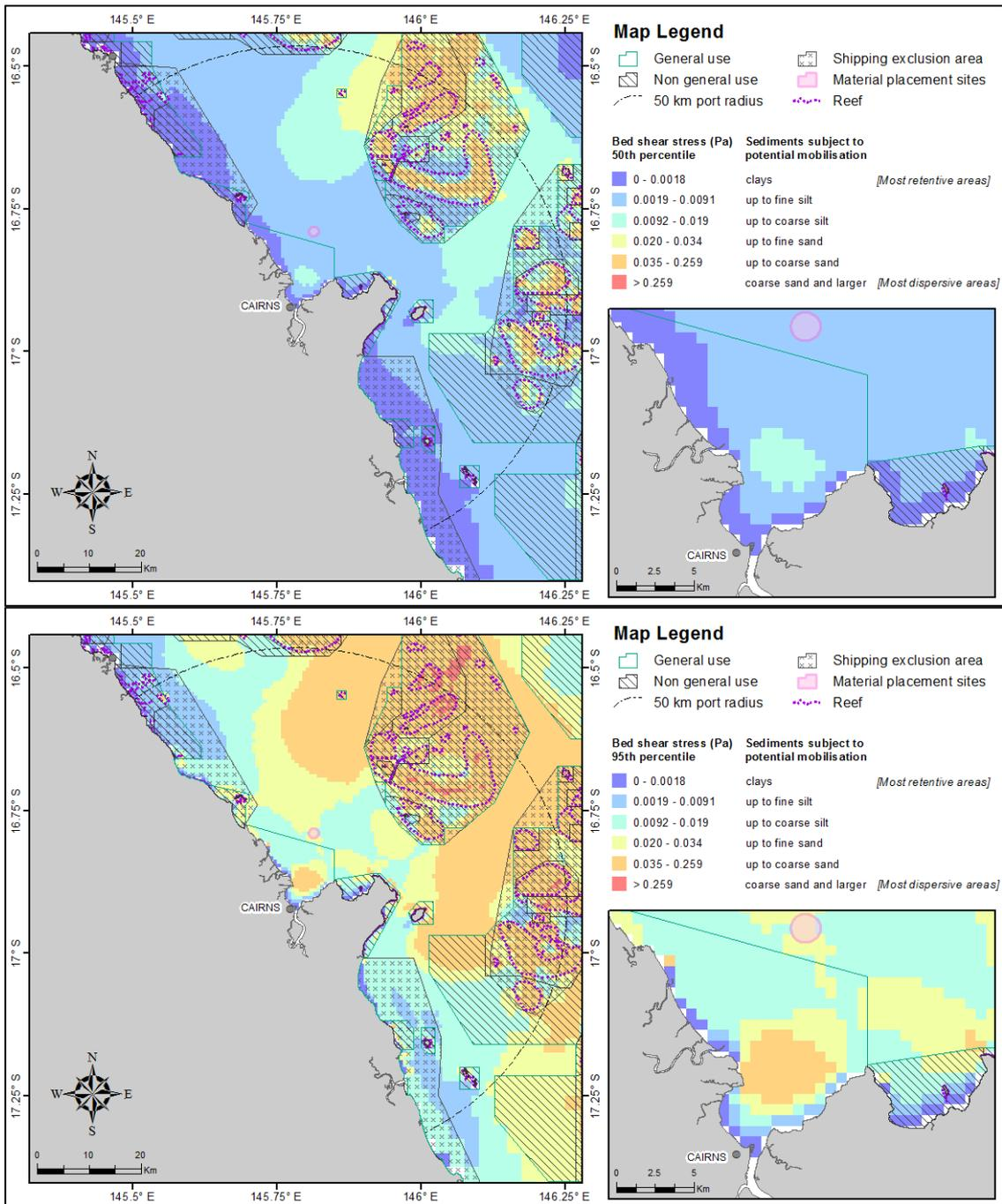
**Figure 43.** Distribution of the 50<sup>th</sup> (upper image) and 95<sup>th</sup> (lower image) percentile bed shear-stress estimates within 50 km from the Port of Cairns. The estimates were calculated at hourly steps for each grid cell during 2011 current and wave conditions. The insets show a close-up view of the bed shear-stress estimates adjacent to the existing disposal site.
