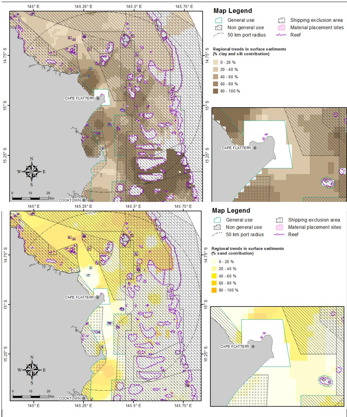
**Figure 48.** Percentage clay-silt (upper image) and sand (lower image) content in surface sediments within 50 km from the Port of Cape Flattery (source: Geoscience Australia marine samples database 2007).
