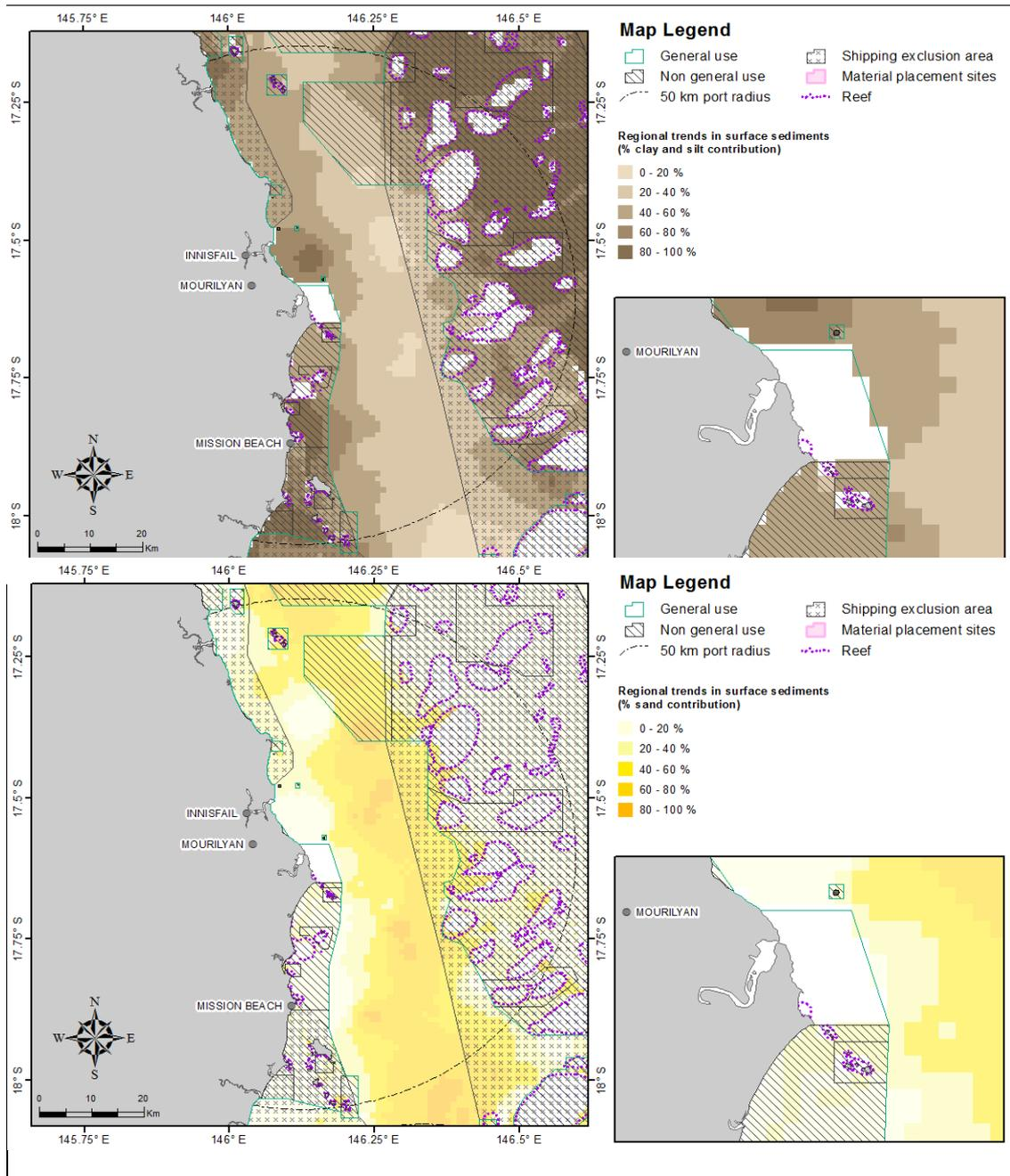
**Figure 42.** Percentage clay-silt (upper image) and sand (lower image) content in surface sediments within 50 km from the Port of Mourilyan (source: Geoscience Australia marine samples database 2007).
