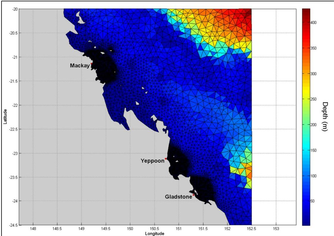
**Figure 16.** Extent of the southern GBR wave model grid. The size of the individual triangles represent the varying mesh resolution and the colour coding the water depth (m).
