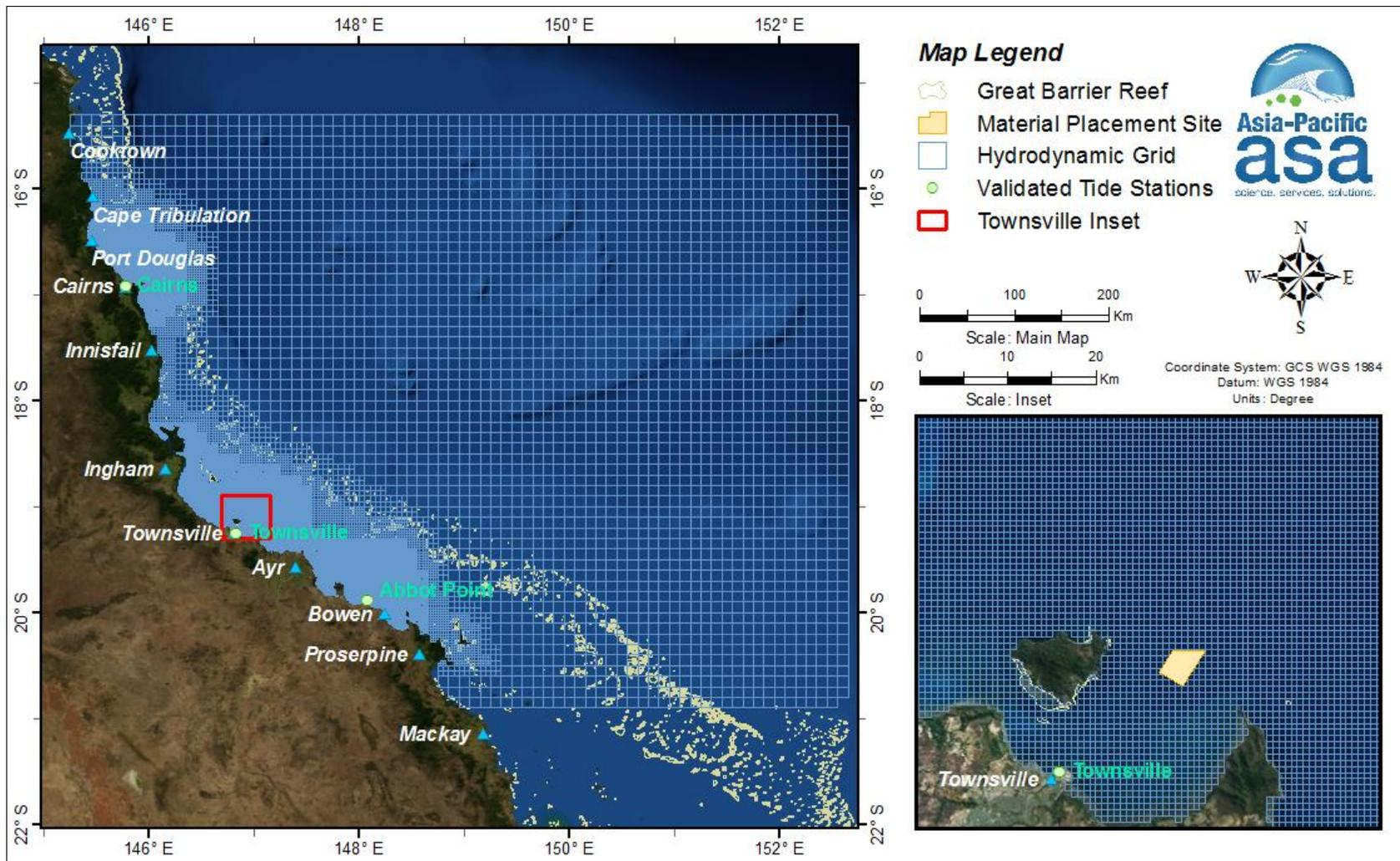
**Figure 7.** Extent of the central GBR coastal model grid. Note the smaller grid cells along the coastline and around islands to recreate the complex flows. The inset shows the smaller grid cells neighbouring Port of Townsville with the yellow box defining the location of the existing dredge material placement site.
