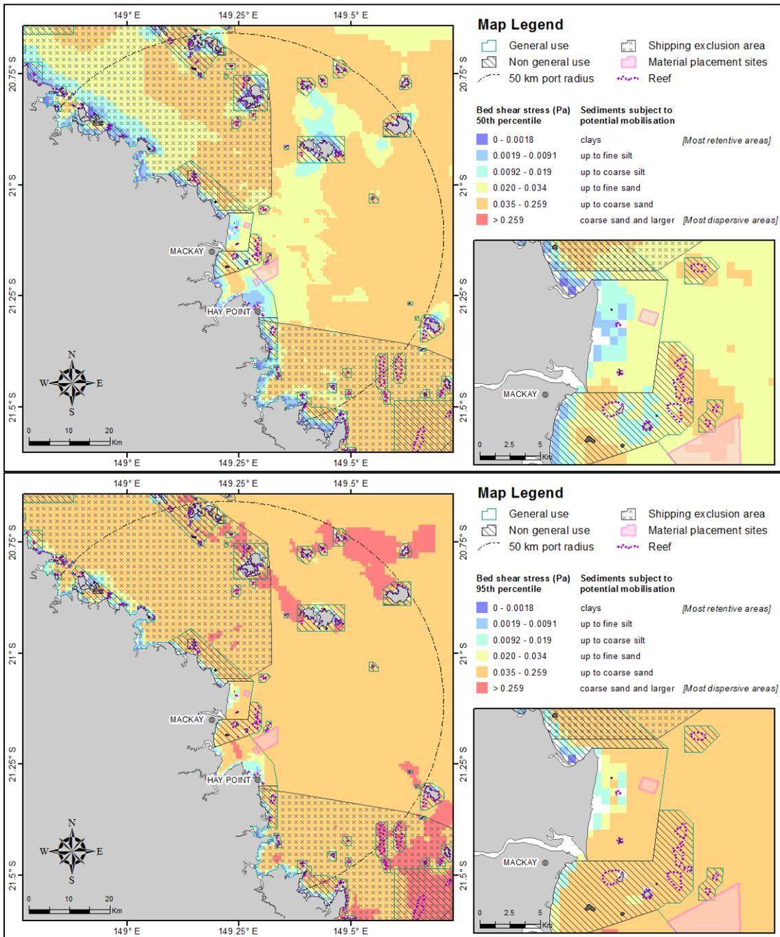
**Figure 33.** Distribution of the 50<sup>th</sup> (upper) and 95<sup>th</sup> (lower image) percentile bed shear-stress estimates within 50 km from the Port of Mackay. The estimates were calculated at hourly steps for each grid cell during 2011 current and wave conditions. The insets show a close-up view of the bed shear-stress estimates adjacent to the existing disposal site.
