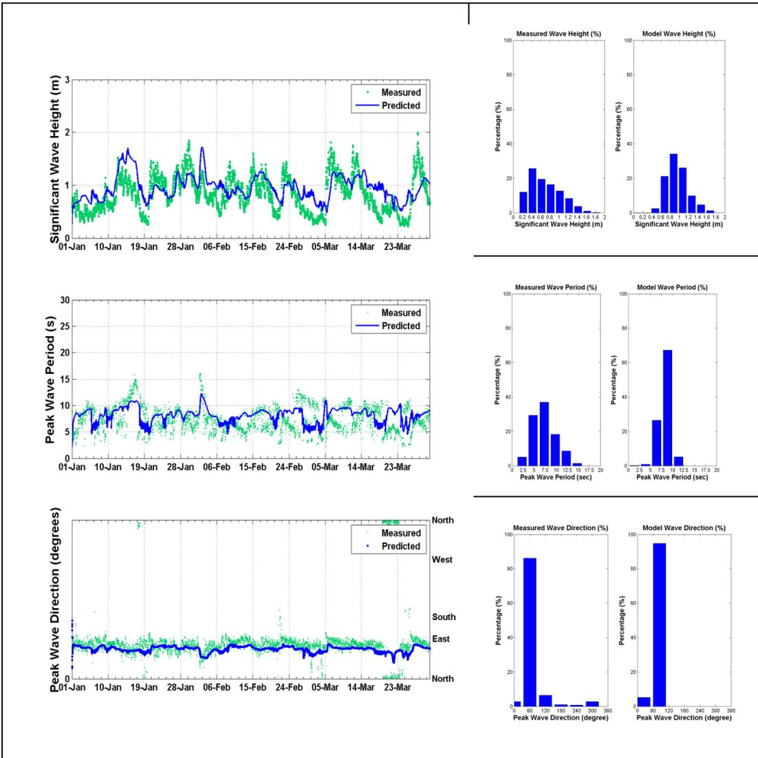
**Figure 21.** Comparison of predicted (blue) and measured (green) waves at the Gladstone waverider buoy, January to March 2011. The top panel shows the significant wave height, the middle panel shows the peak wave period and the bottom panel shows the peak wave direction comparisons. The histograms provide an inter-comparison of the frequency distributions between the observed and predicted.
