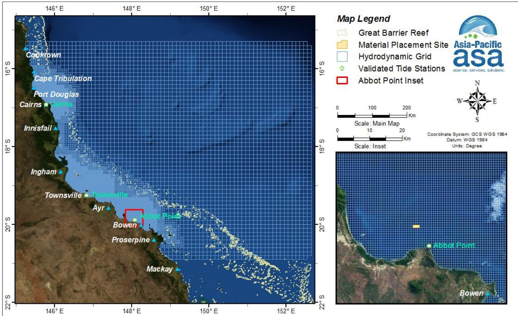
**Figure 6.** Extent of the central GBR coastal model grid. Note the smaller grid cells along the coastline and around islands to recreate the complex flows. The inset shows the smaller grid cells neighbouring Port of Abbot Point with the yellow box defining the location of the existing dredge material placement site.
