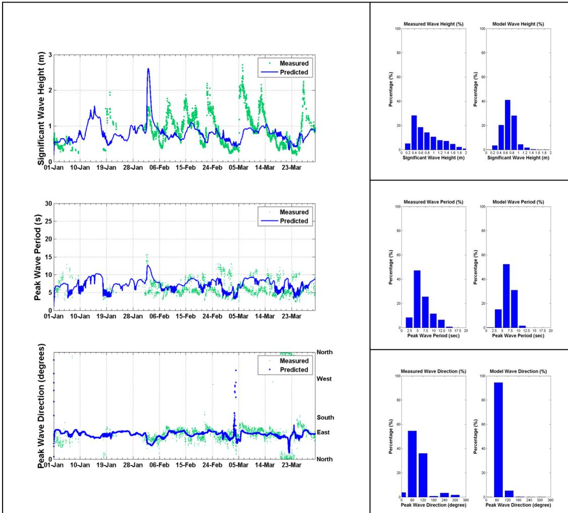
**Figure 22.** Comparison of predicted (blue) and measured (green) waves at the Emu Park waverider buoy, January to March 2011. The top panel shows the significant wave height, the middle panel shows the peak wave period and the bottom panel shows the peak wave direction comparisons. The histograms provide an inter-comparison of the frequency distributions between the observed and predicted.
