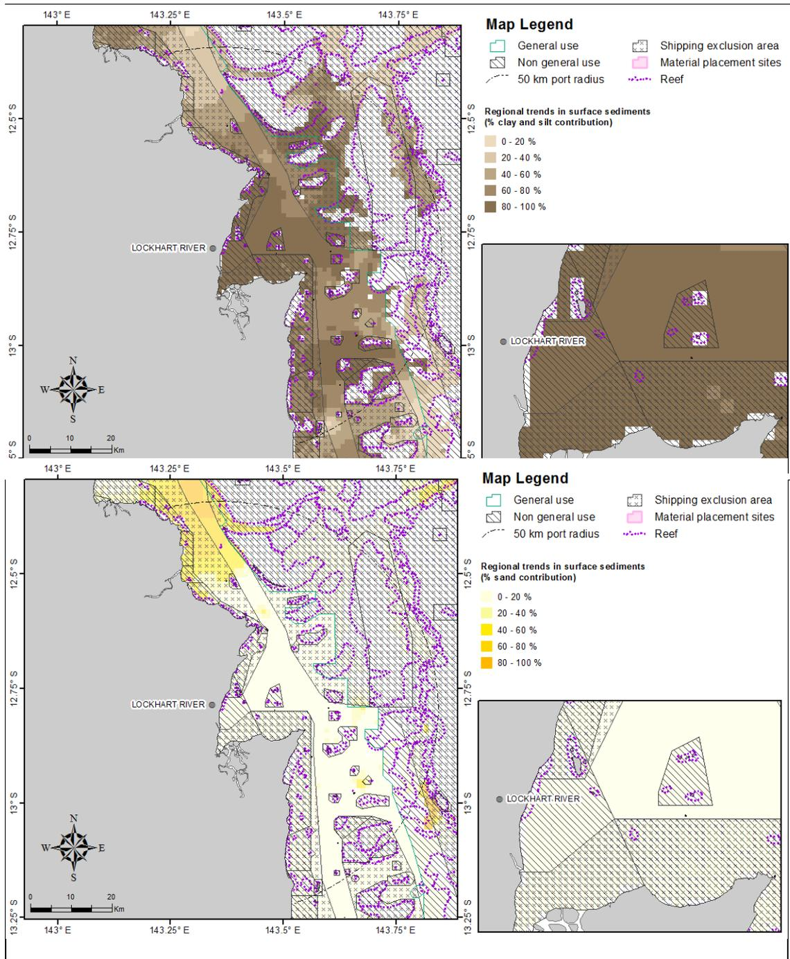
**Figure 50.** Percentage clay-silt (upper image) and sand (lower image) content in surface sediments within 50 km from the Port of Quintell Beach (source: Geoscience Australia marine samples database 2007).
