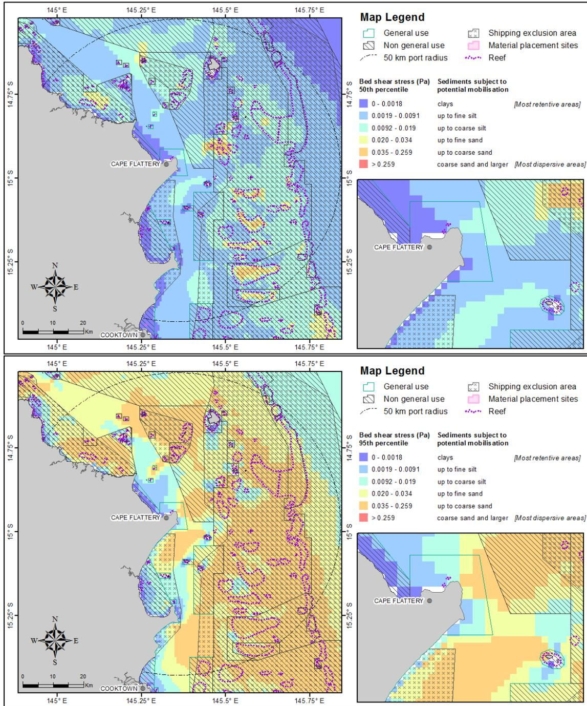
**Figure 47.** Distribution of the 50<sup>th</sup> (upper image) and 95<sup>th</sup> (lower image) percentile bed shear-stress estimates within 50 km from the Port of Cape Flattery. The estimates were calculated at hourly steps for each grid cell during 2011 current and wave conditions. The insets show a close-up view of the bed shear-stress estimates adjacent to the existing disposal site.
