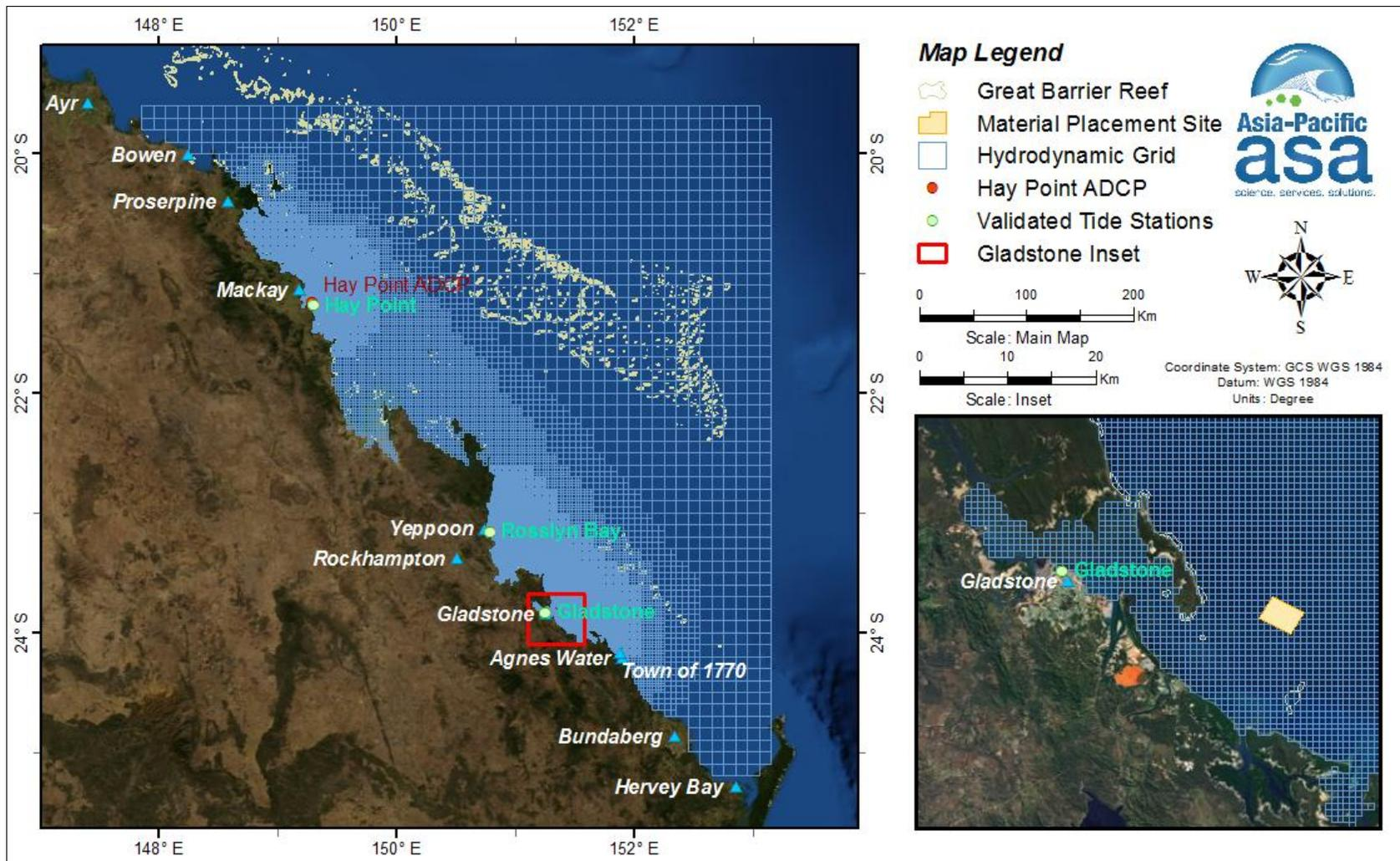
**Figure 3.** Extent of the southern GBR coastal model grid. Note the smaller grid cells along the coastline and around islands to better resolve the complex flows around these features. The inset shows the smaller grid cells neighbouring the Port of Gladstone with the yellow box defining the location of the existing dredge material placement site.
