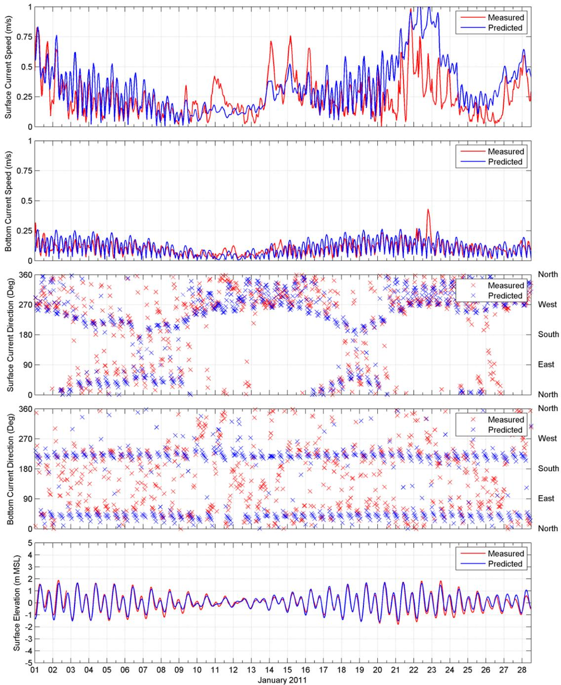
**Figure 15.** Comparison of the predicted and measured surface and bottom current speeds (upper panels) and directions (lower images) and water elevations adjacent to the existing Townsville disposal site (1-29 January 2011).
