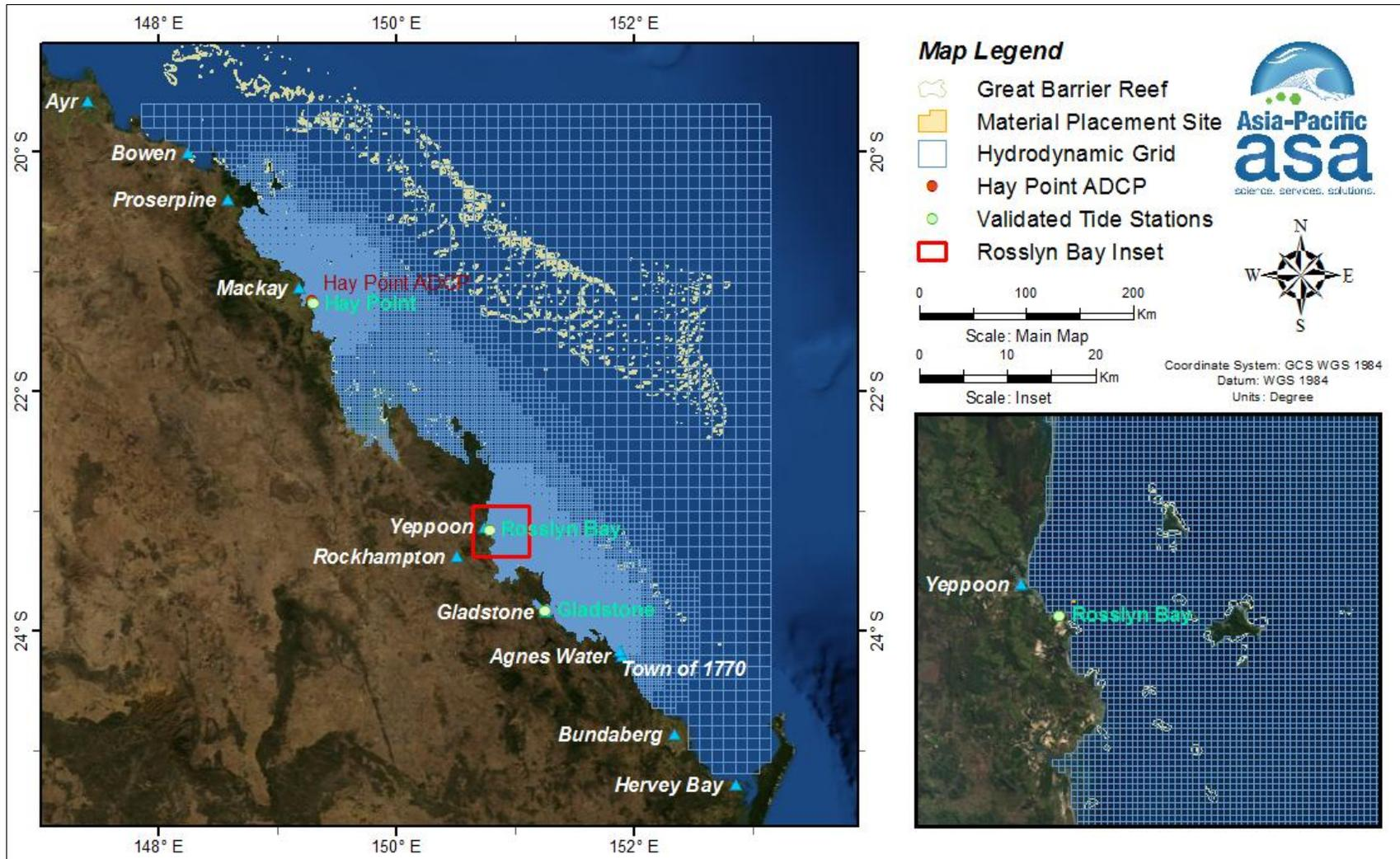
**Figure 4.** Extent of the southern GBR coastal model grid. Note the smaller grid cells along the coastline and around islands to recreate the complex flows. The inset shows the smaller grid cells neighbouring Rosslyn Bay State Boat Harbour with the yellow box defining the location of the existing dredge material placement site.
