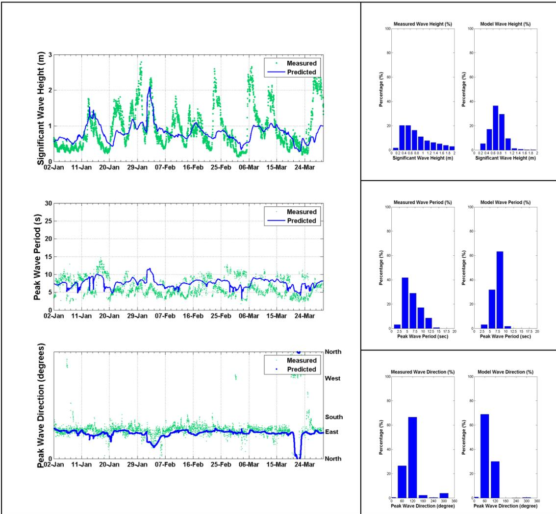
**Figure 23.** Comparison of predicted (blue) and measured (green) waves at the Mackay waverider buoy, January to March 2011. The top panel shows the significant wave height, the middle panel shows the peak wave period and the bottom panel shows the peak wave direction comparisons. The histograms provide an inter-comparison of the frequency distributions between the observed and predicted.
