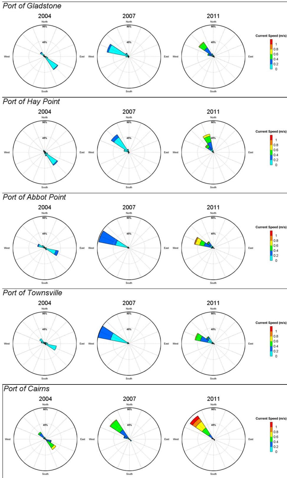
**Figure 2.** Comparative surface current roses for three years adjacent to (from top to bottom) Port of Gladstone, Port of Hay Point, Port of Abbot Point, Port of Townsville and Port of Cairns. The roses cover El Niño (2004), La Niña (2011) and neutral (2007) conditions and are for locations adjacent to the existing material placement sites.
