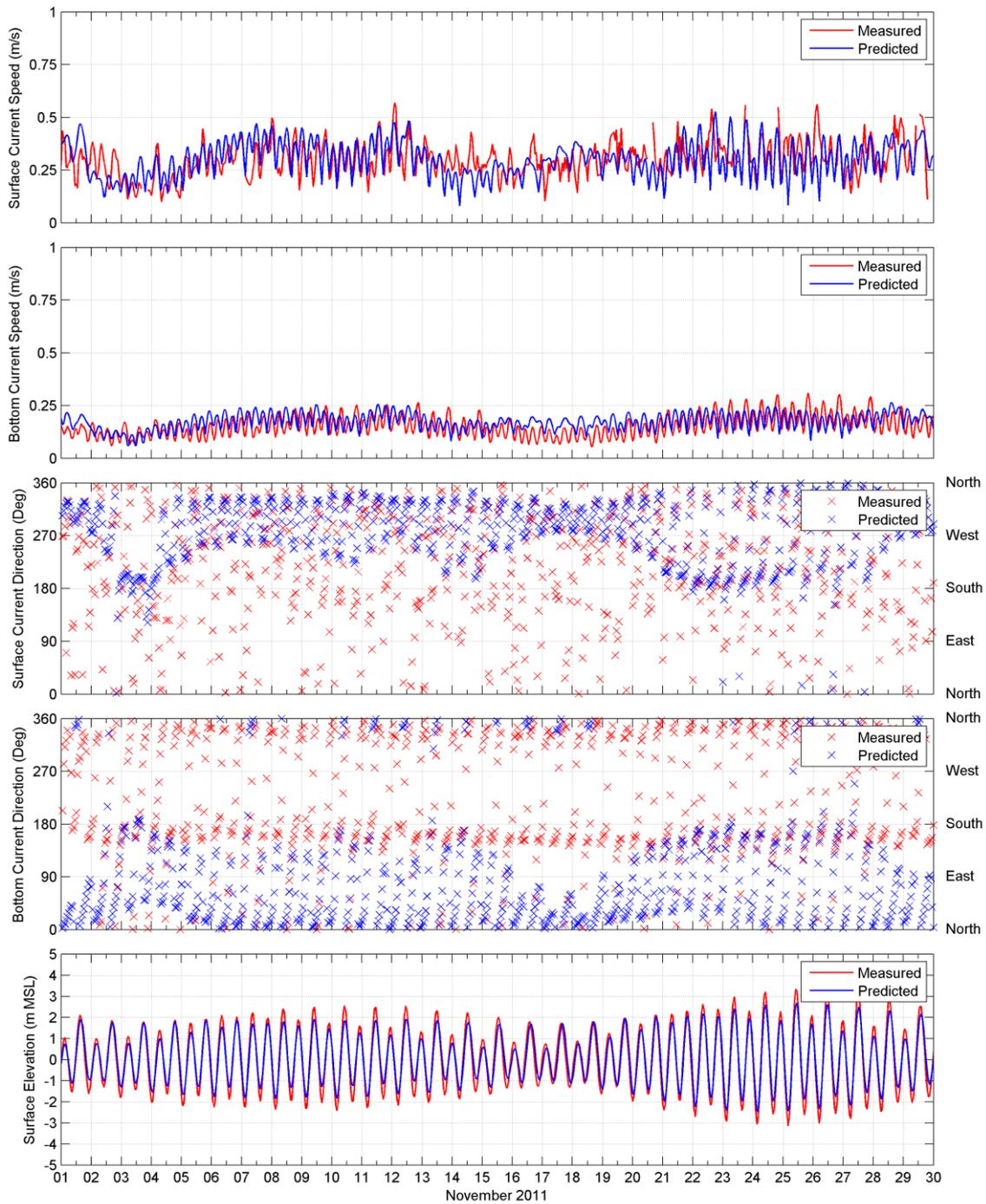
**Figure 14.** Comparison of the predicted and measured surface and bottom current speeds (upper images) and directions (lower images) and water elevations adjacent to the existing Hay Point disposal site (1-30 November 2011).
