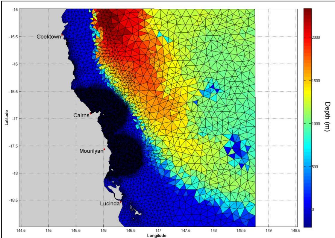
**Figure 18.** Extent of the northern central GBR wave model grid. The size of the individual triangles represent the varying mesh resolution and the colour coding the water depth (m).
