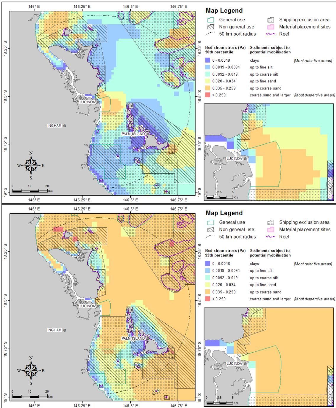
**Figure 39.** Distribution of the 50<sup>th</sup> (upper image) and 95<sup>th</sup> (lower image) percentile bed shear-stress estimates within 50 km from the Port of Lucinda. The estimates were calculated at hourly steps for each grid cell during 2011 current and wave conditions. The insets show a close-up view of the bed shear-stress estimates adjacent to the existing disposal site.
