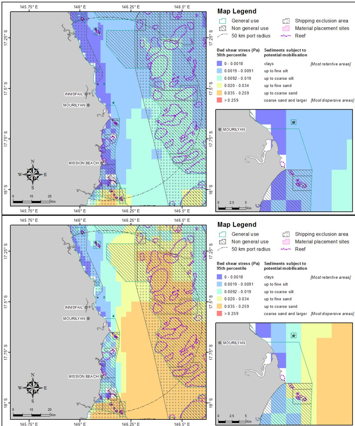
**Figure 41.** Distribution of the 50<sup>th</sup> (upper image) and 95<sup>th</sup> (lower image) percentile bed shear-stress estimates within 50 km from the Port of Mourilyan. The estimates were calculated at hourly steps for each grid cell during 2011 current and wave conditions. The insets show a close-up view of the bed shear-stress estimates adjacent to the existing disposal site.
