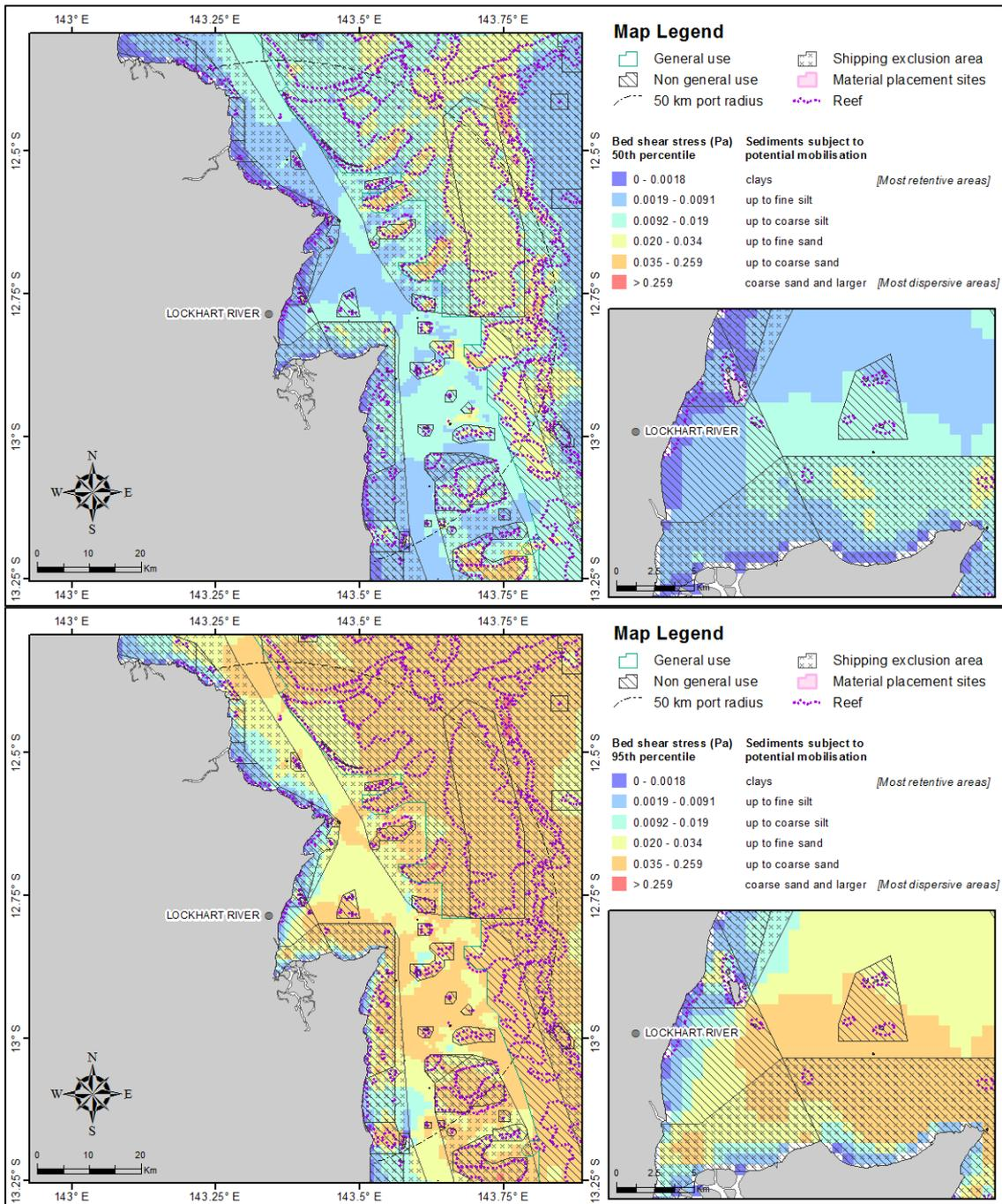
**Figure 49.** Distribution of the 50<sup>th</sup> (upper image) and 95<sup>th</sup> (lower image) percentile bed shear-stress estimates within 50 km from the Port of Quintell Beach. The estimates were calculated at hourly steps for each grid cell during 2011 current and wave conditions. The insets show a close-up view of the bed shear-stress estimates adjacent to the existing disposal site.
