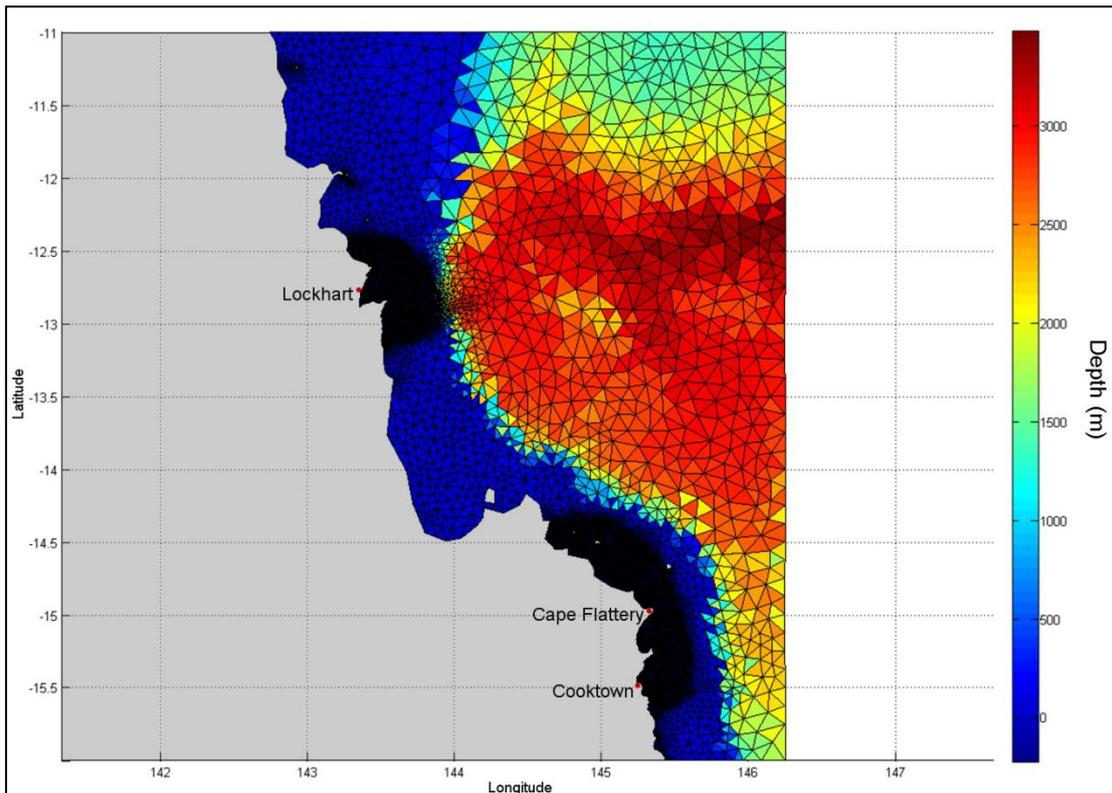
**Figure 19.** Extent of the northern GBR wave model grid. The size of the individual triangles represent the varying mesh resolution and the colour coding the water depth (m).
