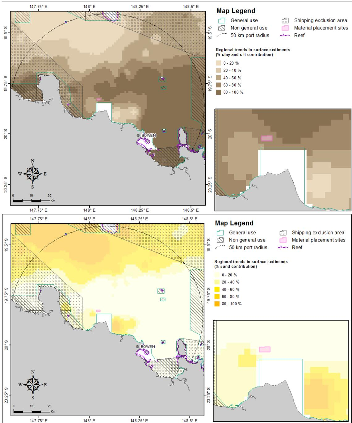
**Figure 36.** Percentage for clay-silt (upper image) and sand (lower image) content in surface sediments within 50 km from the Port of Abbot Point (source Geoscience Australia marine samples database 2007).
