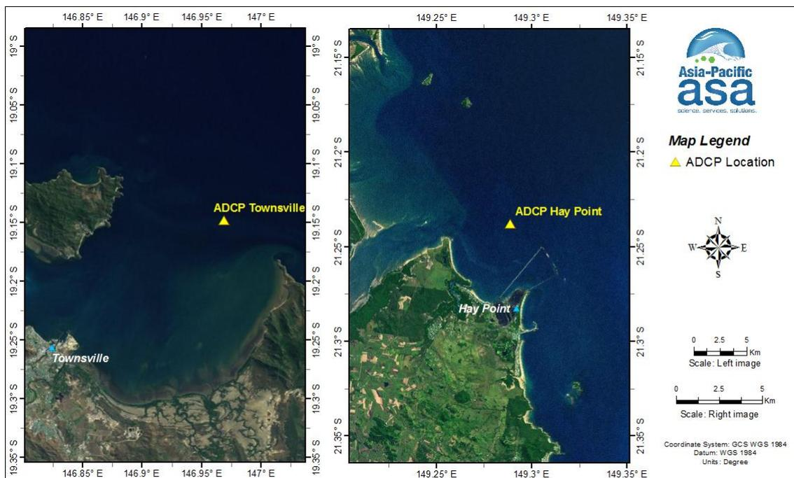
**Figure 13.** Locations of the bottom mounted Acoustic Doppler Current Profilers (ADCPs) instruments used to measure currents throughout water column adjacent to the Townsville and Hay Point existing material placement sites in January and November 2011, respectively.
