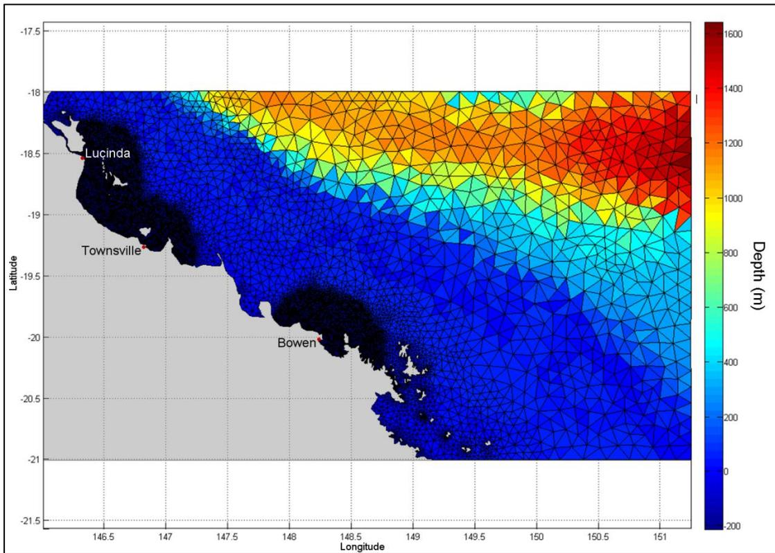
**Figure 17.** Extent of the southern central GBR wave model grid. The size of the individual triangles represent the varying mesh resolution and the colour coding the water depth (m).
