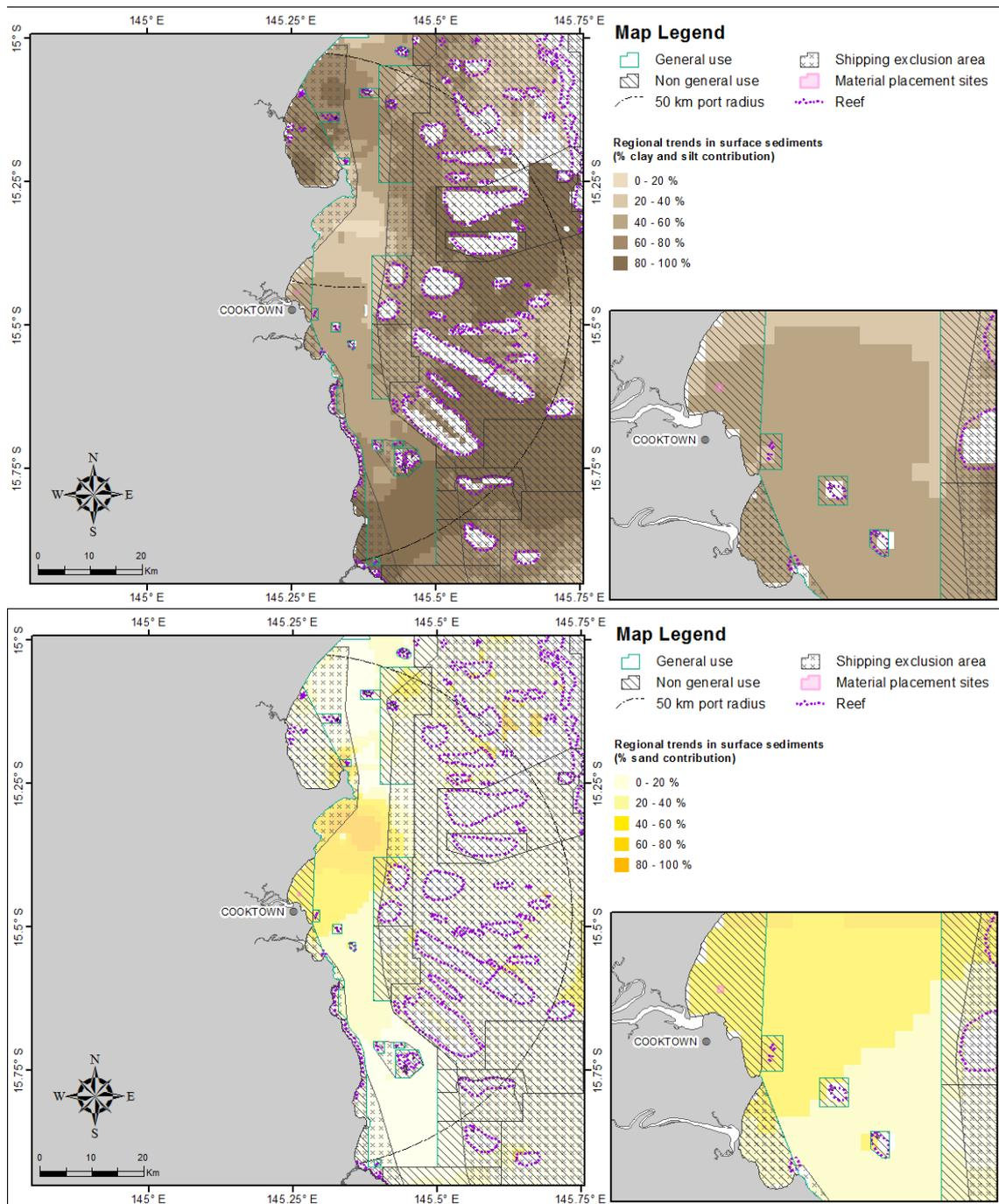
**Figure 46.** Percentage clay-silt (upper image) and sand (lower image) content in surface sediments within 50 km from the Port of Cooktown (source: Geoscience Australia marine samples database 2007).
