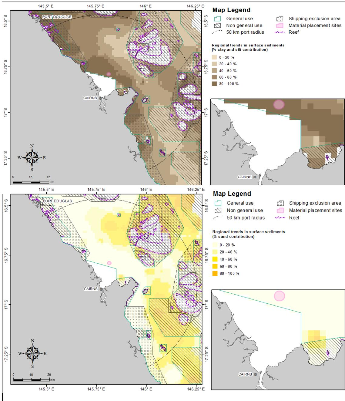
**Figure 44.** Percentage clay-silt (upper image) and sand (lower image) content in surface sediments within 50 km from the Port of Cairns (source: Geoscience Australia marine samples database 2007).
