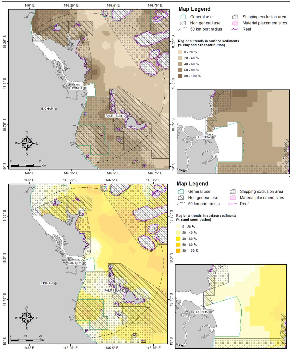
**Figure 40.** Percentage clay-silt (upper image) and sand (lower image) content in surface sediments within 50 km from the Port of Lucinda (source: Geoscience Australia marine samples database 2007).
