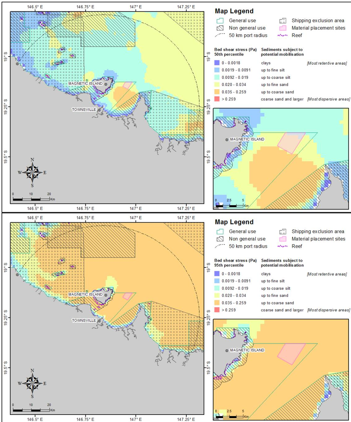
**Figure 37.** Distribution of the 50<sup>th</sup> (upper) and 95<sup>th</sup> (lower image) percentile bed shear-stress estimates within 50 km from the Port of Townsville. The estimates were calculated at hourly steps for each grid cell during 2011 current and wave conditions. The insets show a close-up view of the bed shear-stress estimates adjacent to the existing disposal site.
