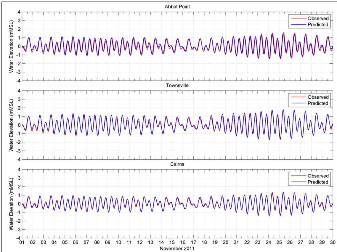
**Figure 11.** Comparison between the predicted (red line) and observed (blue line) water elevations at Abbot Point (upper image), Townsville (middle image) and Cairns (lower image), 1-30 November 2011.
