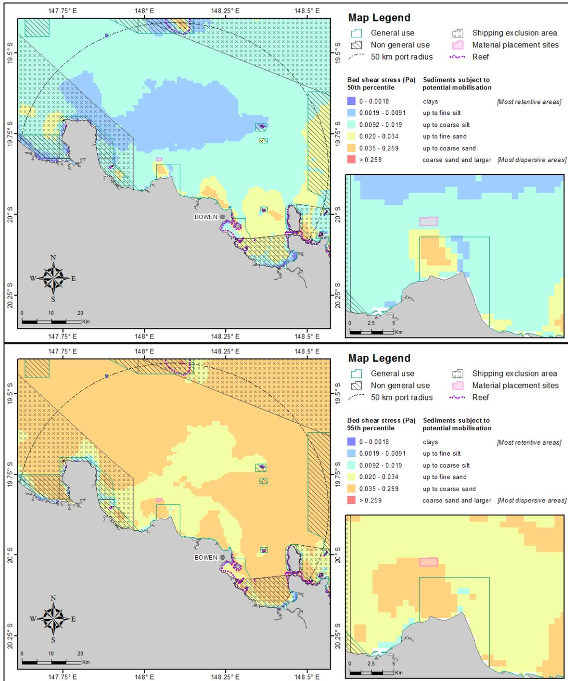
**Figure 35.** Distribution of the 50<sup>th</sup> (upper) and 95<sup>th</sup> (lower image) percentile bed shear-stress estimates within 50 km from the Port of Abbot Point. The estimates were calculated at hourly steps for each grid cell during 2011 current and wave conditions. The insets show a close-up view of the bed shear-stress estimates adjacent to the existing disposal site.
