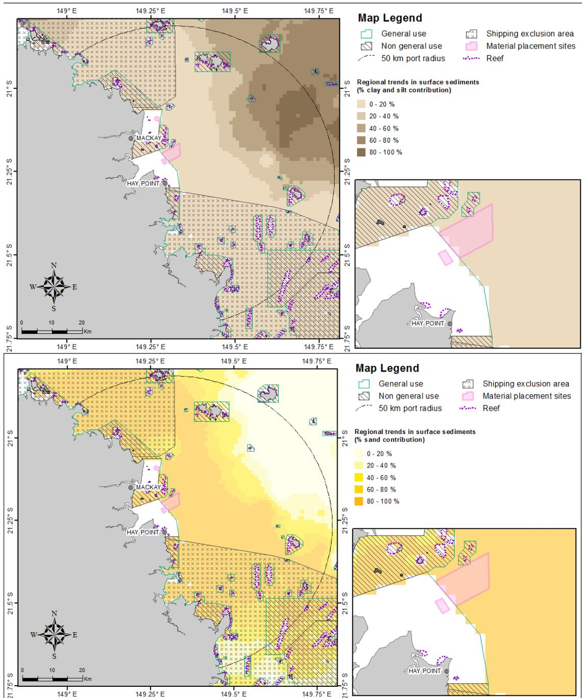
**Figure 32.** Percentage for clay-silt (upper image) and sand (lower image) content in surface sediments within 50 km from the Port of Hay Point (source: Geoscience Australia marine samples database 2007).
