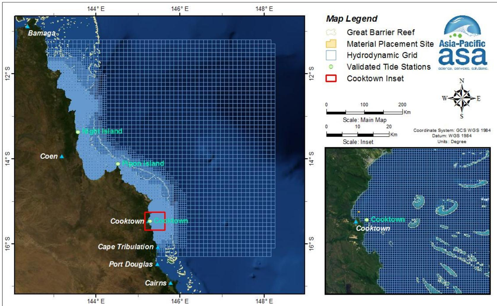
**Figure 9.** Extent of the northern GBR coastal model grid. Note the smaller grid cells along the coastline and around islands to recreate the complex flows. The inset shows the smaller grid cells neighbouring Port of Cooktown with the yellow box defining the location of the existing dredge material placement site.
