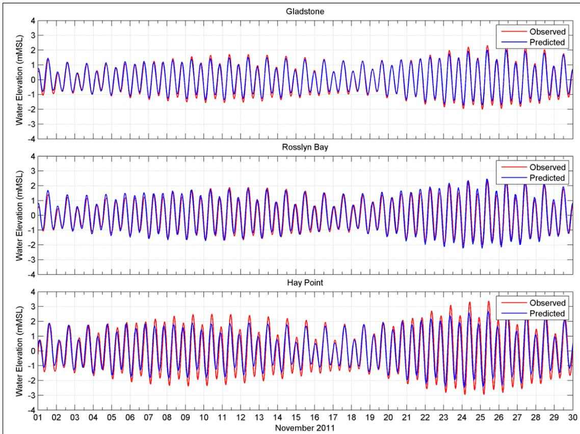
**Figure 10.** Comparison between the predicted (red line) and observed (blue line) water elevations at Gladstone (upper image), Rosslyn Bay (middle image) and Hay Point (lower image), 1-30 November 2011.
