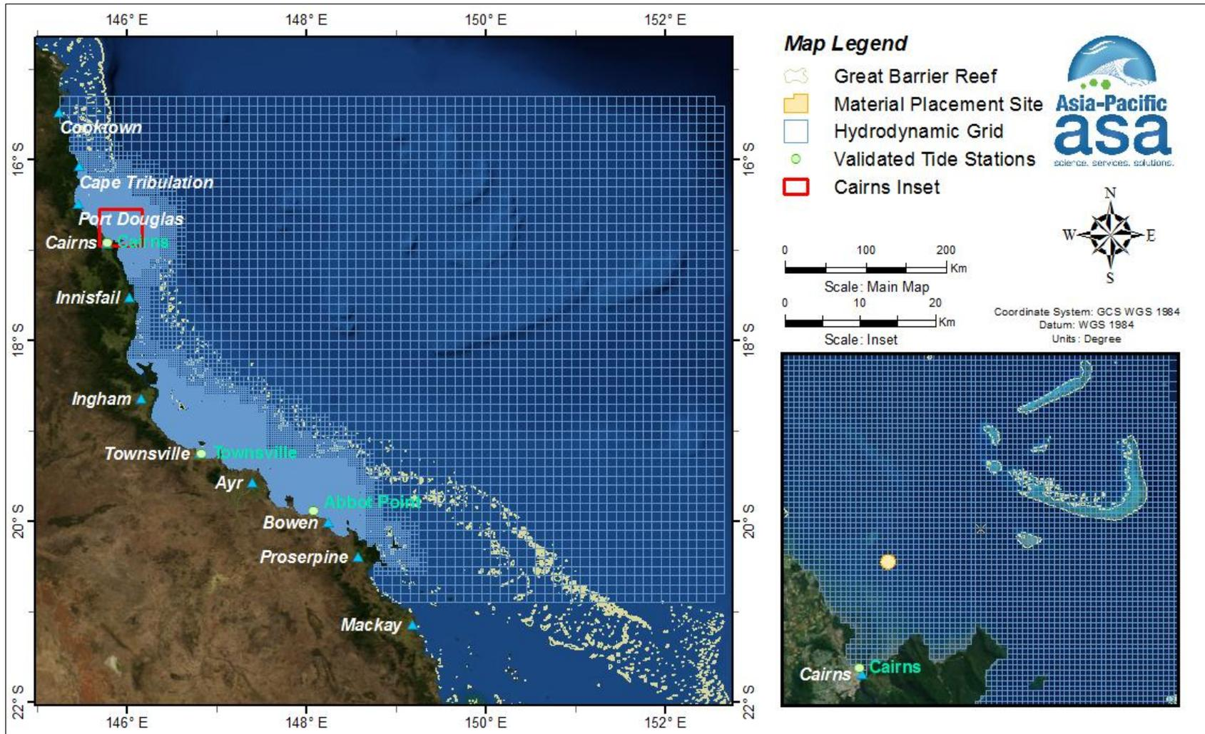
**Figure 8.** Extent of the central GBR coastal model grid. Note the smaller grid cells along the coastline and around islands to recreate the complex flows. The inset shows the smaller grid cells neighbouring Port of Cairns with the yellow box defining the location of the existing dredge material placement site.
