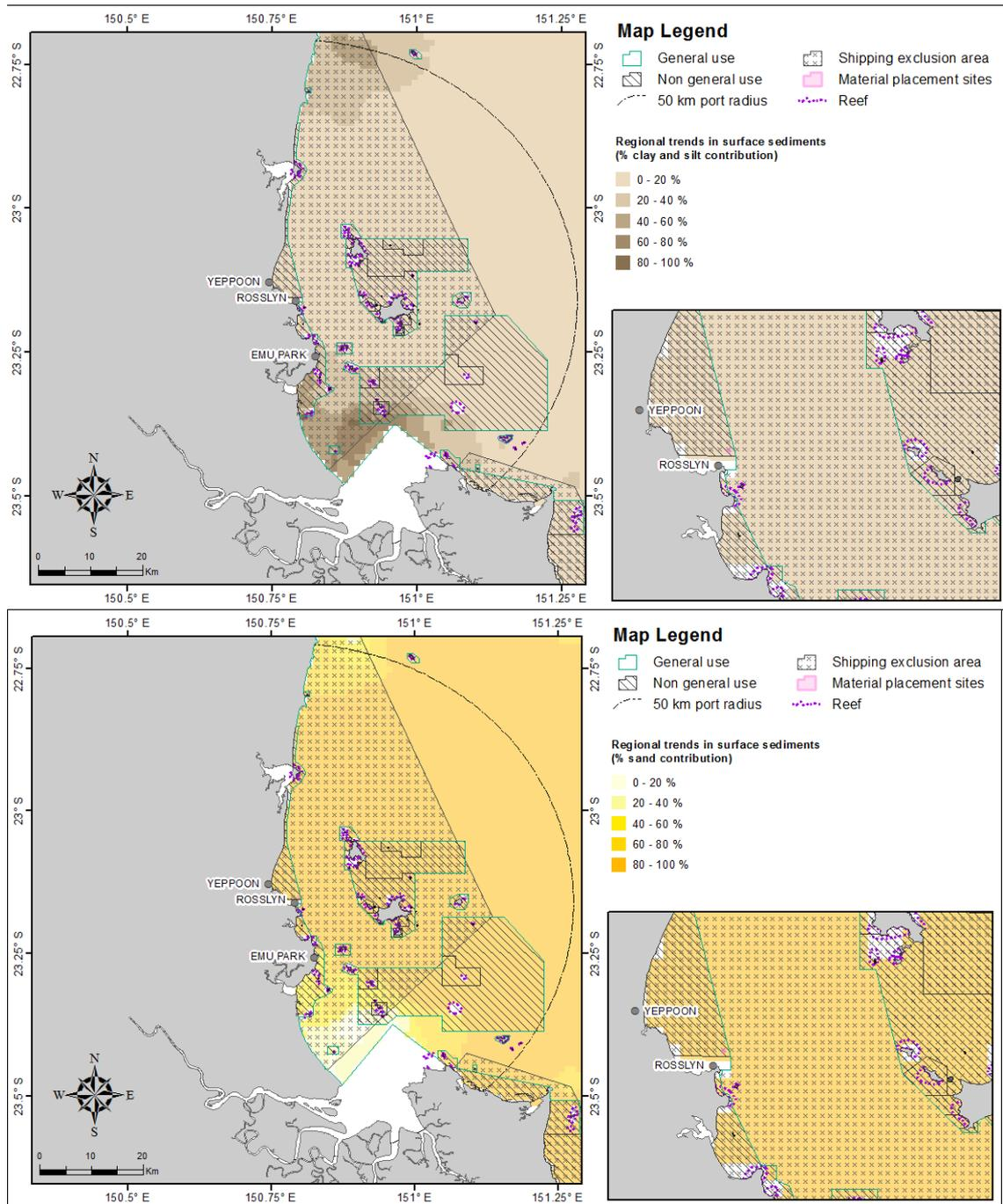
**Figure 30.** Percentage for clay-silt (upper image) and sand (lower image) content in surface sediments within 50 km from Rosslyn Bay State Boat Harbour (source: Geoscience Australia marine samples database 2007).
