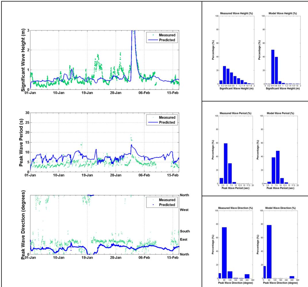
**Figure 24.** Comparison of predicted (blue) and measured (green) waves at the Townsville waverider buoy, January to February 2011. The top panel shows the significant wave height, the middle panel shows the peak wave period and the bottom panel shows the peak wave direction comparisons. The histograms provide an inter-comparison of the frequency distributions between the observed and predicted.
