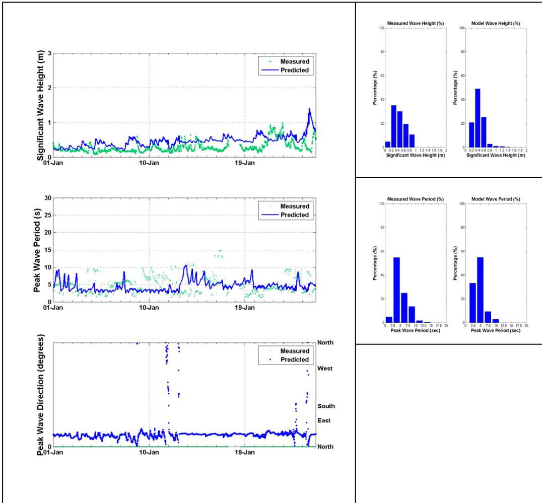
**Figure 25.** Comparison of predicted (blue) and measured (green) waves at the Cairns waverider buoy, January to February 2011. The top panel shows the significant wave height and the bottom panel shows the peak wave period. The histograms provide an inter-comparison of the frequency distributions between the observed and predicted.
