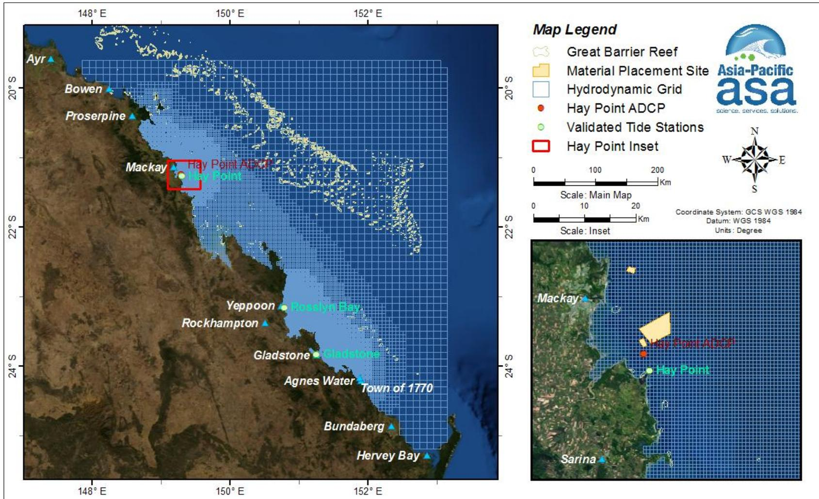
**Figure 5.** Extent of the southern GBR coastal model grid. Note the smaller grid cells along the coastline and around islands to recreate the complex flows. The inset shows the smaller grid cells neighbouring Port of Hay Point with the yellow box defining the location of the existing dredge material placement site.
