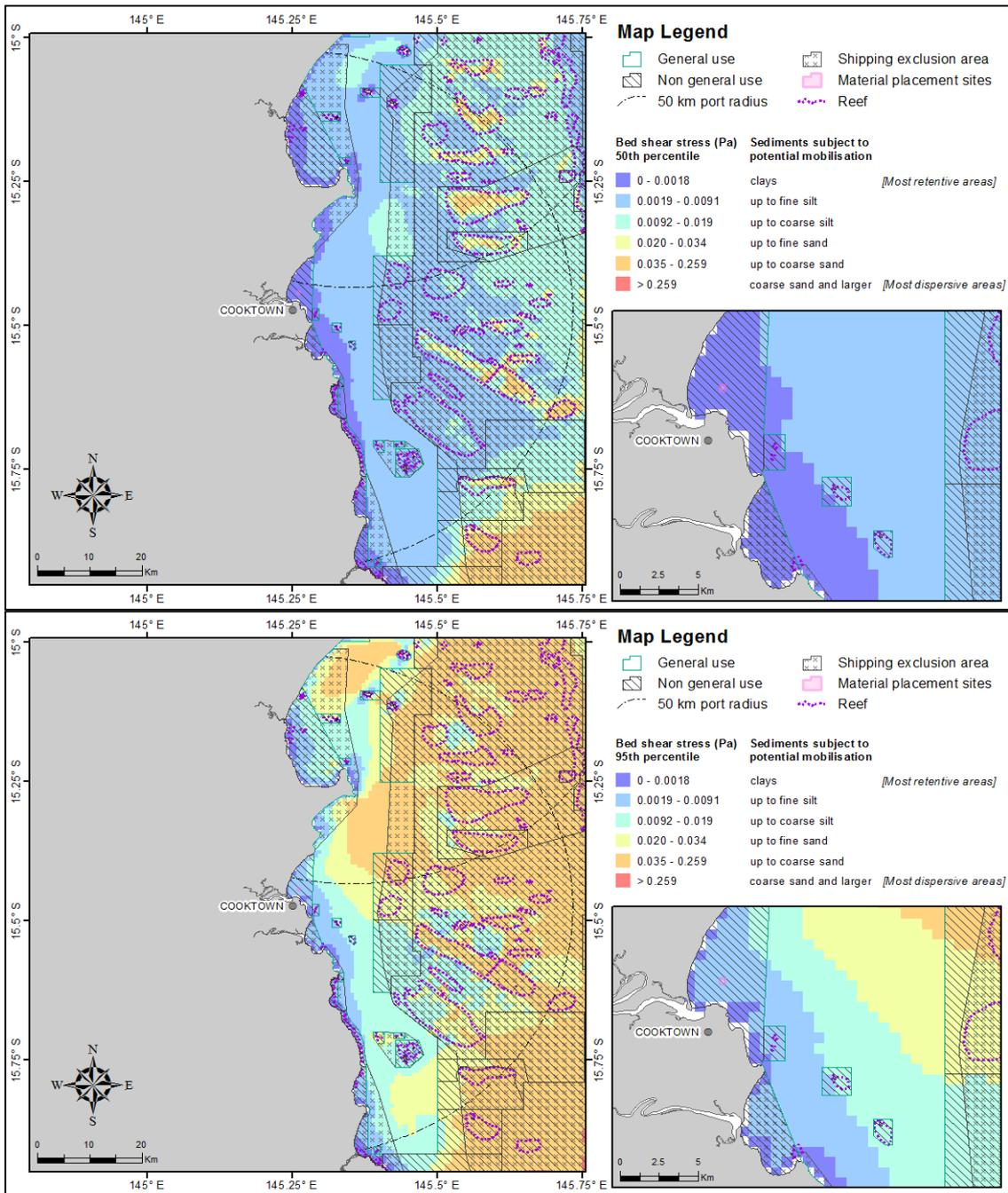
**Figure 45.** Distribution of the 50<sup>th</sup> (upper image) and 95<sup>th</sup> (lower image) percentile bed shear-stress estimates within 50 km from the Port of Cooktown. The estimates were calculated at hourly steps for each grid cell during 2011 current and wave conditions. The insets show a close-up view of the bed shear-stress estimates adjacent to the existing disposal site.
