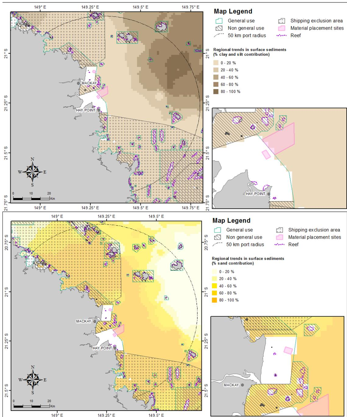
**Figure 34.** Percentage for clay-silt (upper image) and sand (lower image) content in surface sediments within 50 km from the Port of Mackay (source: Geoscience Australia marine samples database 2007).
