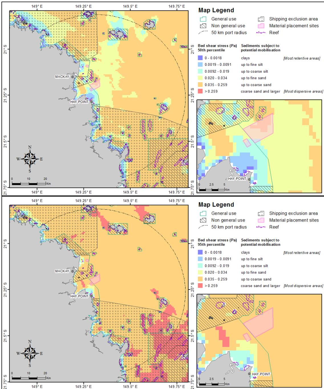
**Figure 31.** Distribution of the 50<sup>th</sup> (upper) and 95<sup>th</sup> (lower image) percentile bed shear-stress estimates within 50 km from the Port of Hay Point. The estimates were calculated at hourly steps for each grid cell during 2011 current and wave conditions. The insets show a close-up view of the bed shear-stress estimates adjacent to the existing disposal site.
