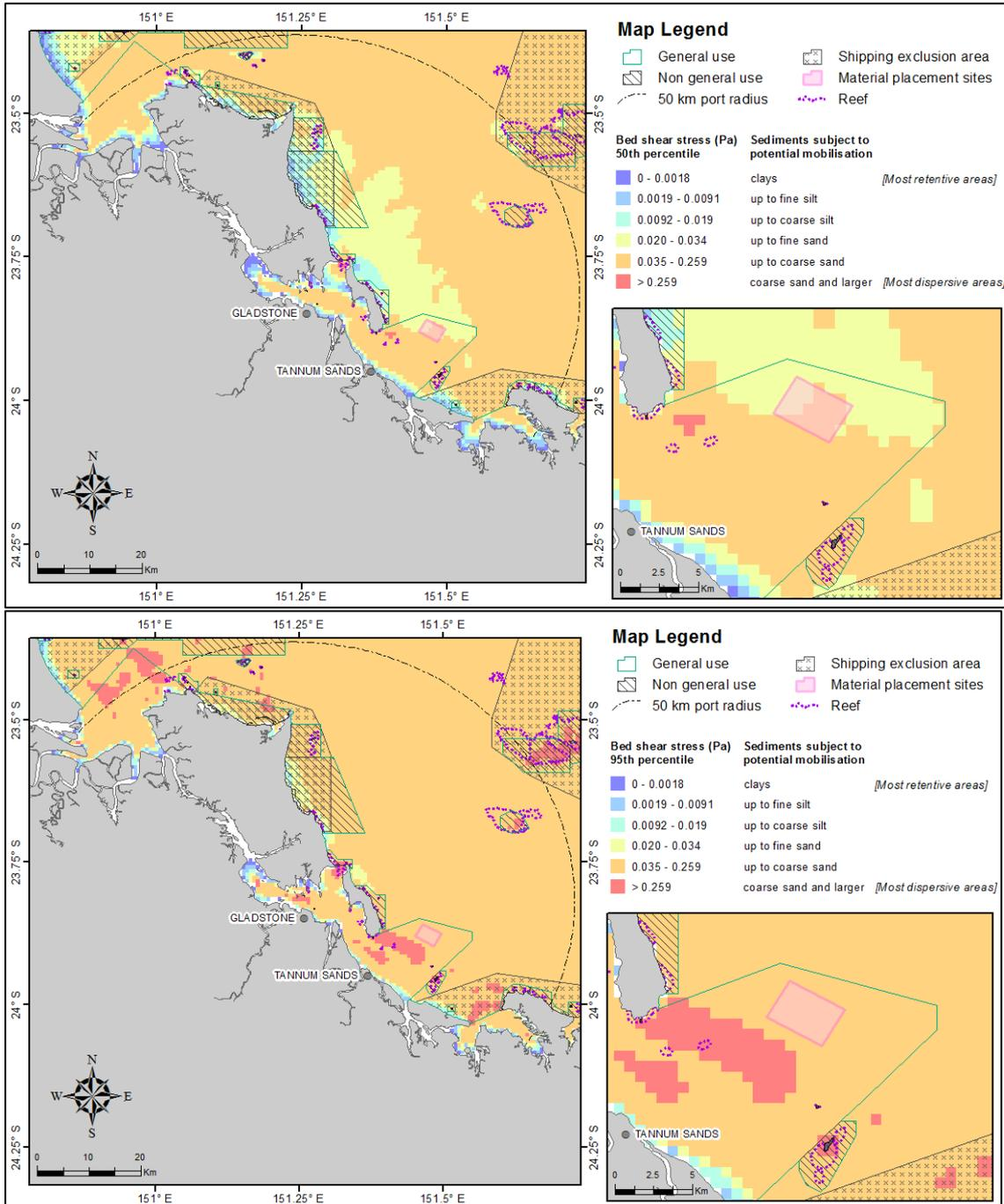
**Figure 27.** Distribution of the 50<sup>th</sup> (upper image) and 95<sup>th</sup> (lower image) percentile bed shear-stress estimates within 50 km from the Port of Gladstone. The estimates were calculated at hourly steps for each grid cell during 2011 current and wave conditions. The insets show a close-up view of the bed shear-stress estimates adjacent to the existing disposal site.
