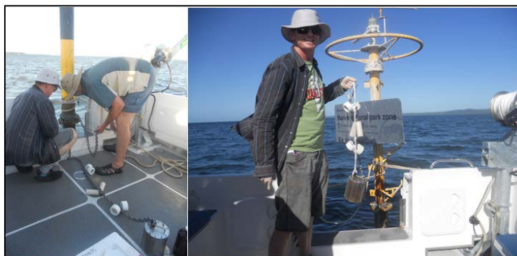
Figure 3 Deployment of passive samplers in the field
