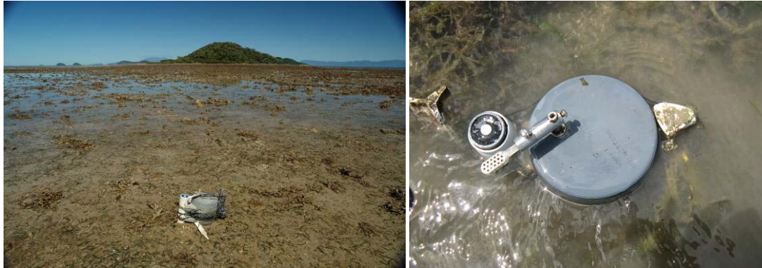
Submersible Odyssey™ photosynthetic irradiance autonomous loggers deployed at Dunk Island (left) and Cockle Bay (right).
