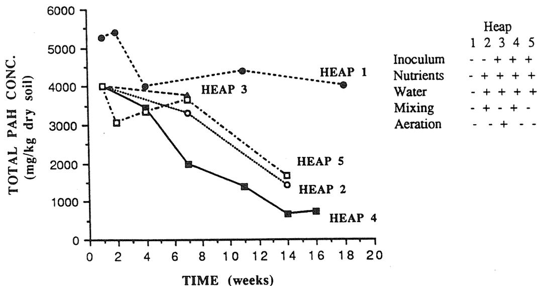
Figure 1. Biodegradation of PAHs in 5 tonne soil heaps
