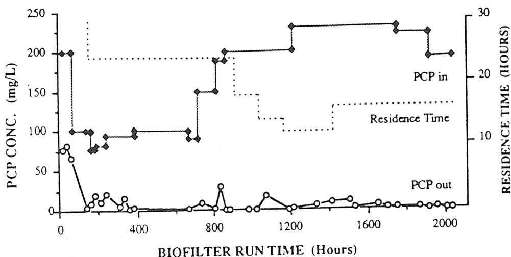
Figure 2. Biodegradation of pentachlorophenol (PCP) in a biofilter.
